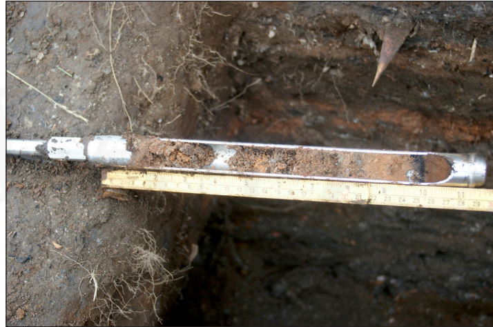
Figure 6. SVB13 Group 08 Soil Core Test made below finishing levels, Southwest corner
