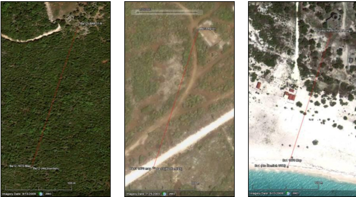
Figure 19. Discrepancy between stations with coordinates from Ato Kentish, with manually measured coordinates from 1970 maps and the location of same stations in Google Earth. Be12 at Highland House left, Be13 at All in Well centre and Ba1 at Martello Tower right. (Photo FSI/Google Earth.)
