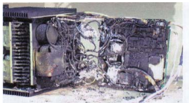
Figure 13. View with the bridge control logic PCB pulled away from the inverter case assembly
