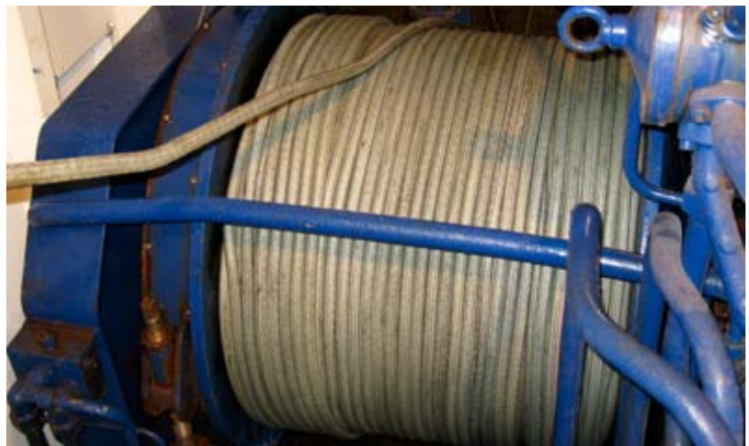
915 metres of 22mm Dynex Warp on Claudia's trawl drums
