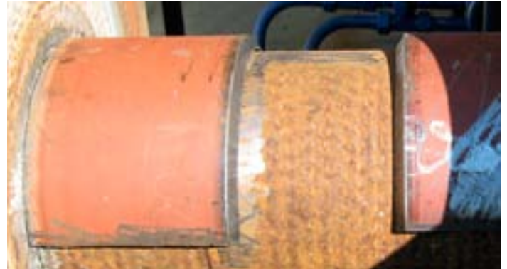
Plates added to strengthen Claudia's winches
