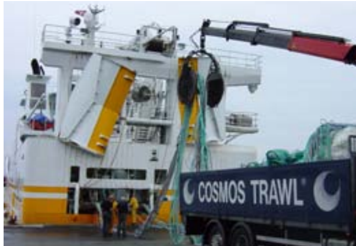
The crew of Isafold haul the new 1024 m Gloria Helix trawl onto the netdrum.
