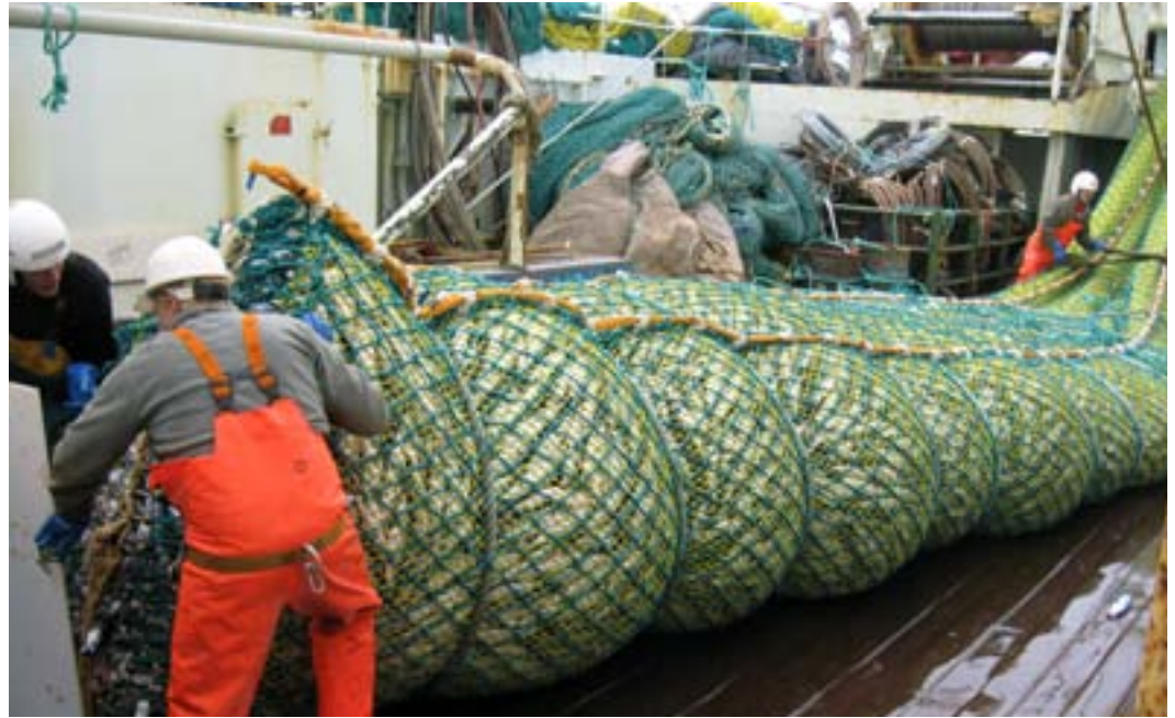
Therney's T90 codend with 10-15 tonnes of mackerel, enough for processing and freezing in six hours.
