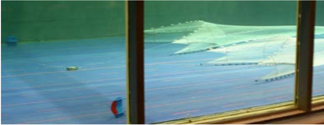
A model of Fjardanet's 3000-mesh twin-rig shrimp trawl in the flume tank in Hirtshals, towed on three warps with a middle clump.
