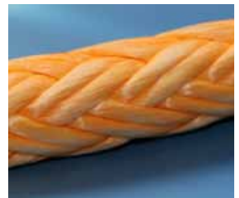
Dynex Dux rope. Pre-tensioning this rope increases the strength by 15% and also reduces the diameter and elongation.
