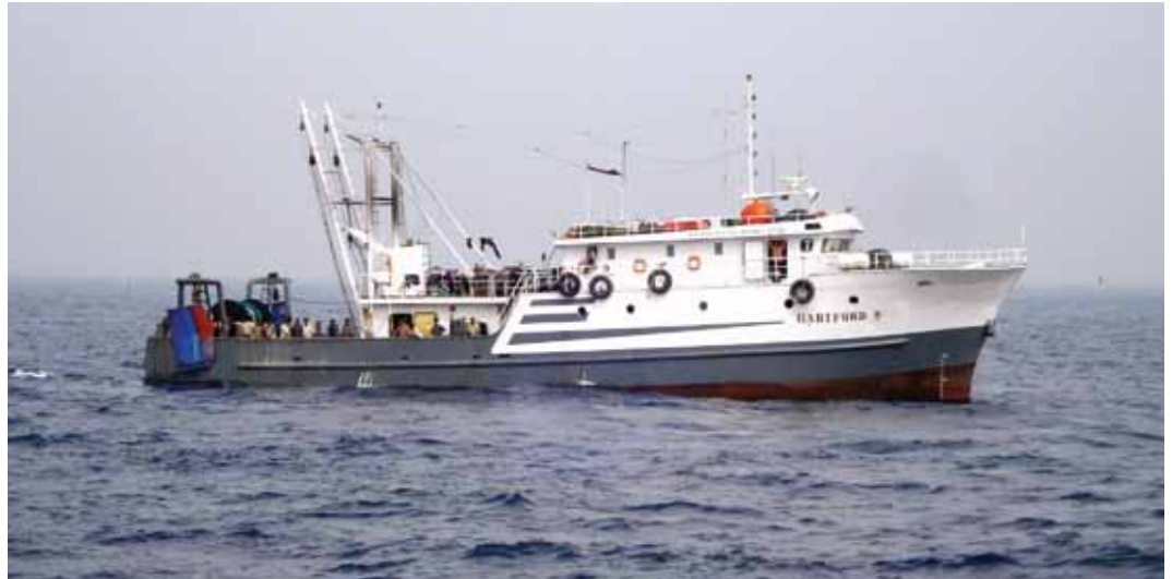
A typical Bangladeshi trawler. The derricks aft are used for shrimp trawling on shallow grounds.
