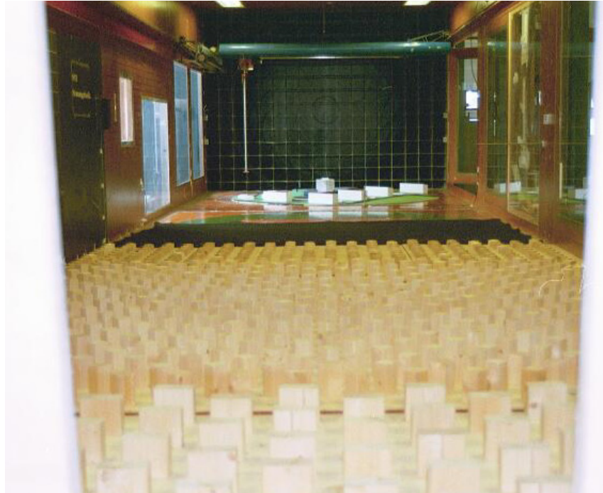
Figure 3.1 The roughness elements and the model of the building and its surroundings, a view from behind the spires downstream in the tunnel looking towards the turntable.
