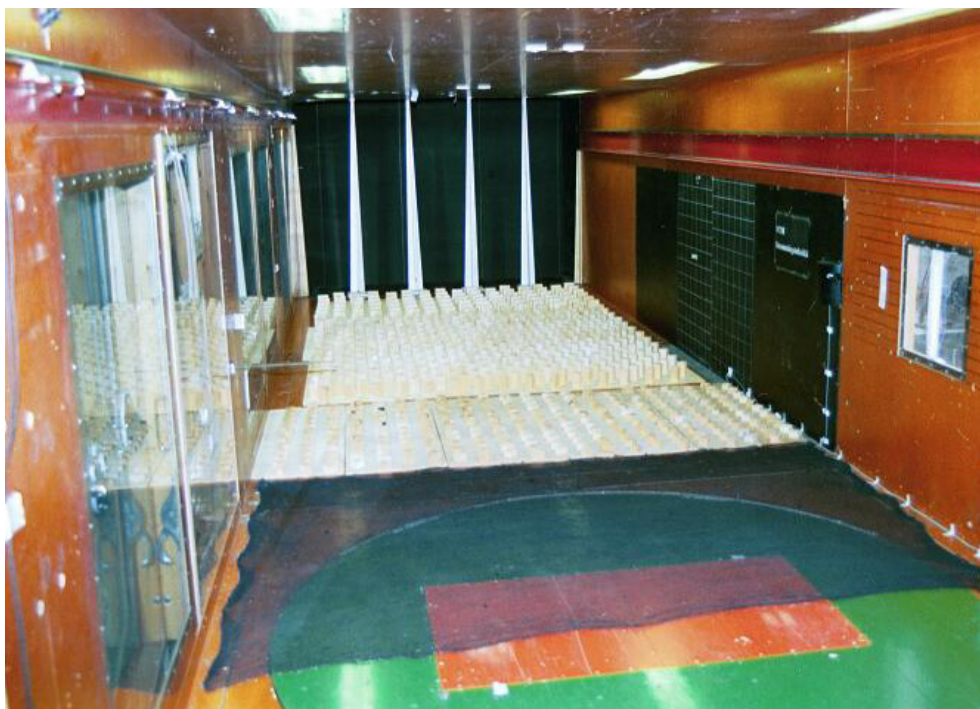
Figure 3.2 The spires and the roughness elements as seen from the turntable.
