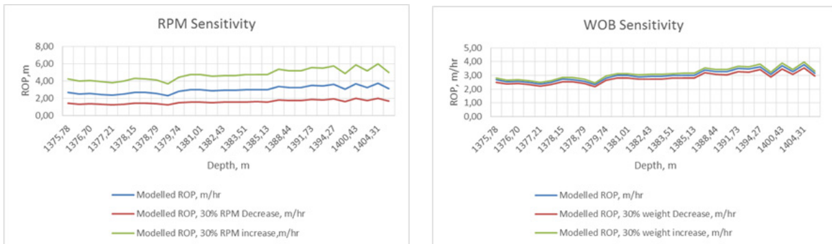
FIGURE 26: Sensitivity of ROP on WOB and RPM for the production hole
