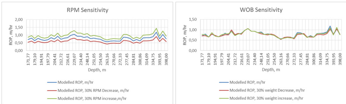
FIGURE 23: Sensitivity of ROP on WOB and RPM for the intermediate hole
