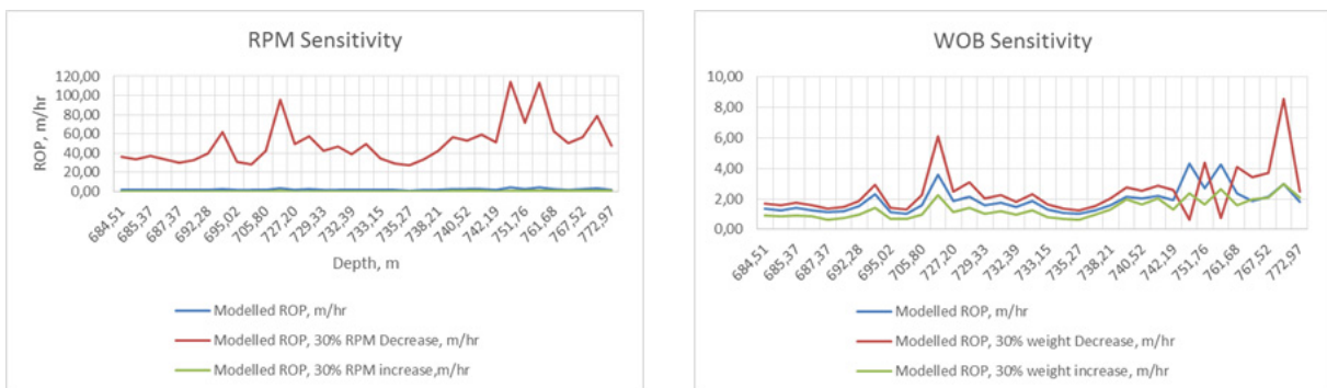
FIGURE 24: Sensitivity of ROP on WOB and RPM for the production hole
