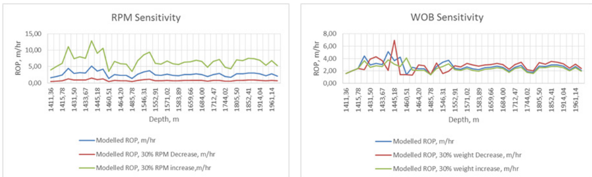
FIGURE 27: Sensitivity of ROP on WOB and RPM for the production hole
