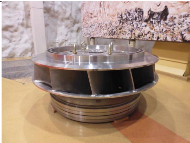
Photo 29: Blanda power station spare runner
