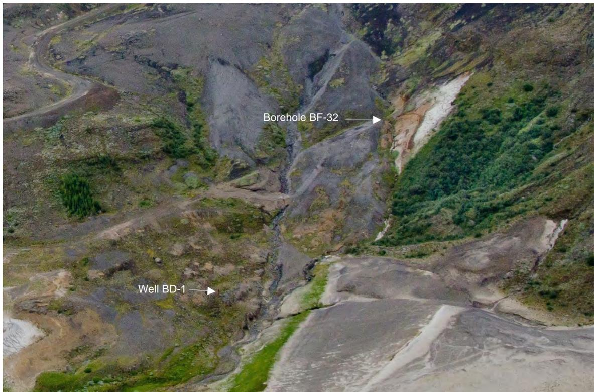
Figure 7-10 Enlargement of part of Figure 7-9. Well BD-1 is located roughly at the middle of proposed surface powerhouse. Borehole BF-32 is roughly 50 m east of station 0+300 along the proposed penstock and on top of glacial till. Photo: Emil Þór Sigurðsson 16 August 2012.
