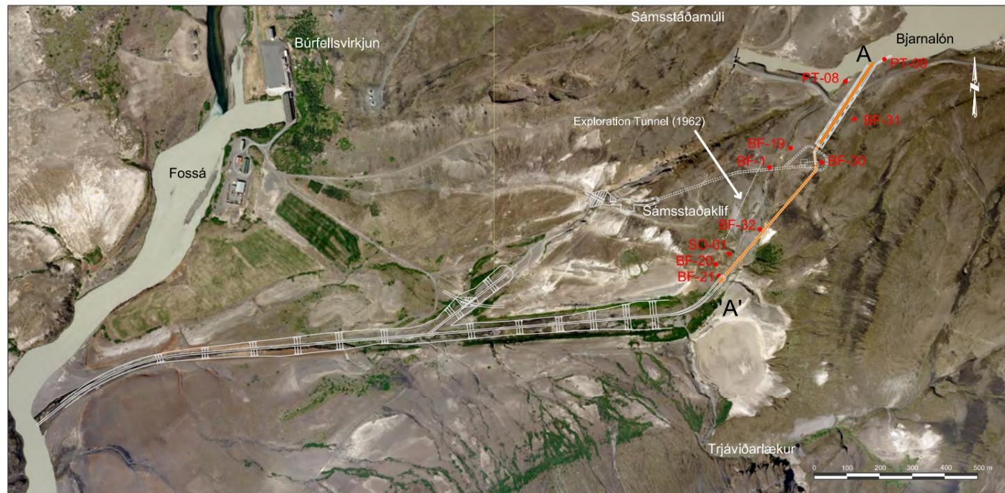
Planview of section and boreholes for Underground Powerhouse alternative
