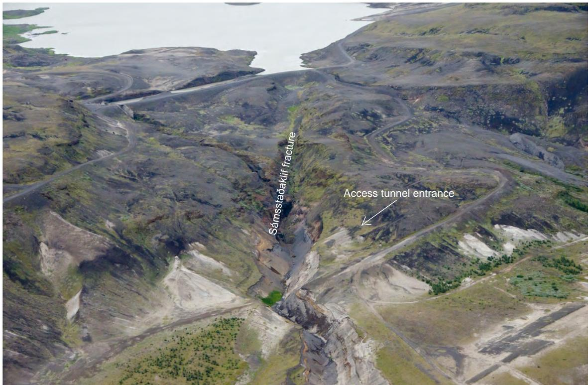
Figure 6-6 Sámstaðaklif-fracture meeting the headrace-canal of Búrfell Station in the centre. Location of access tunnel entrance for Búrfell Extension – Underground alternative. Photo: Emil Þór Sigurðsson 16 August 2012.
