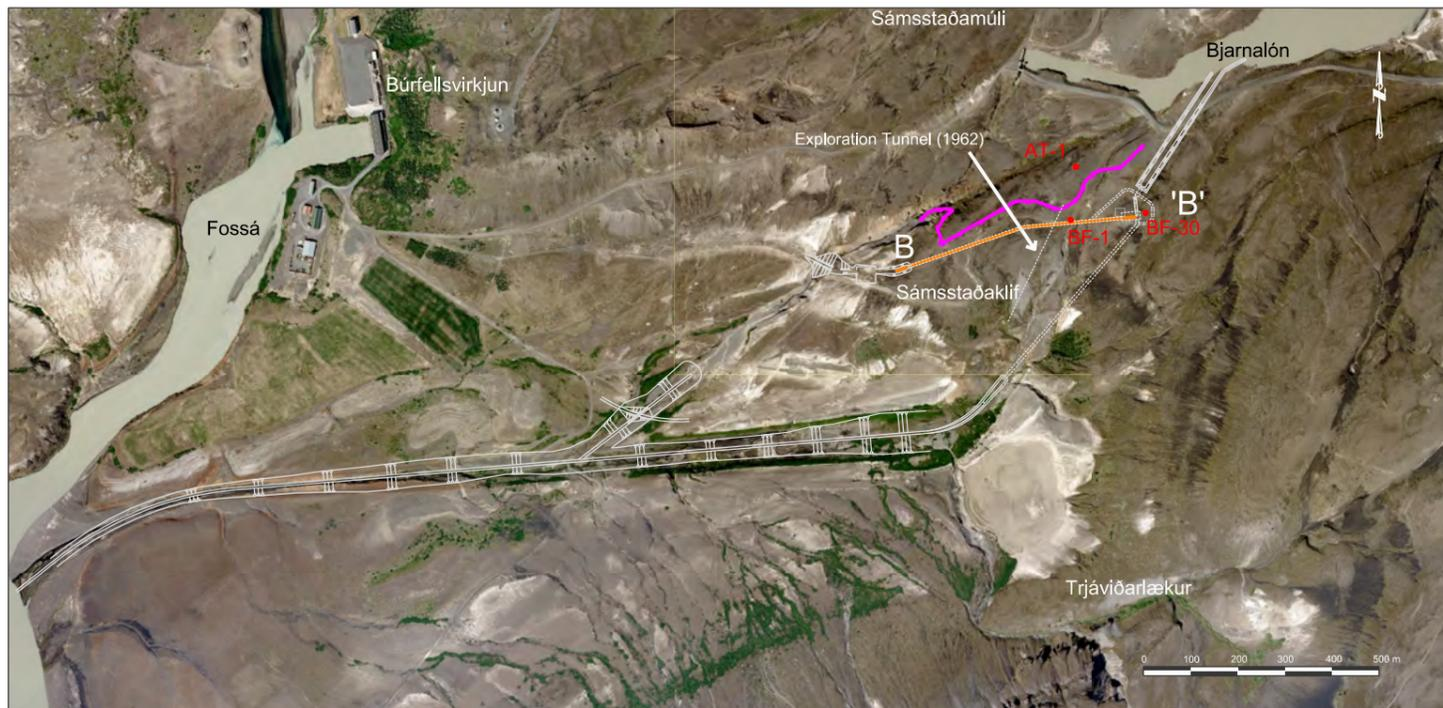
Planview of section and boreholes in Underground Powerhouse alternative
