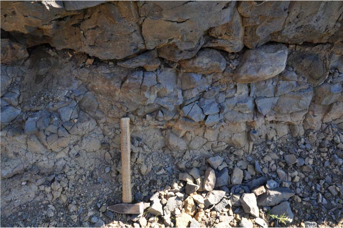
Figure 7-6 Bottom of the section of the trench in Figure 7-6 showing the conglomerate layer underneath the tholeiite basalt seen in borehole BF-19 at elevation 237 m a.s.l. to 239 m a.s.l. Photo: Snorri P. Snorrason 10 July 2012.
