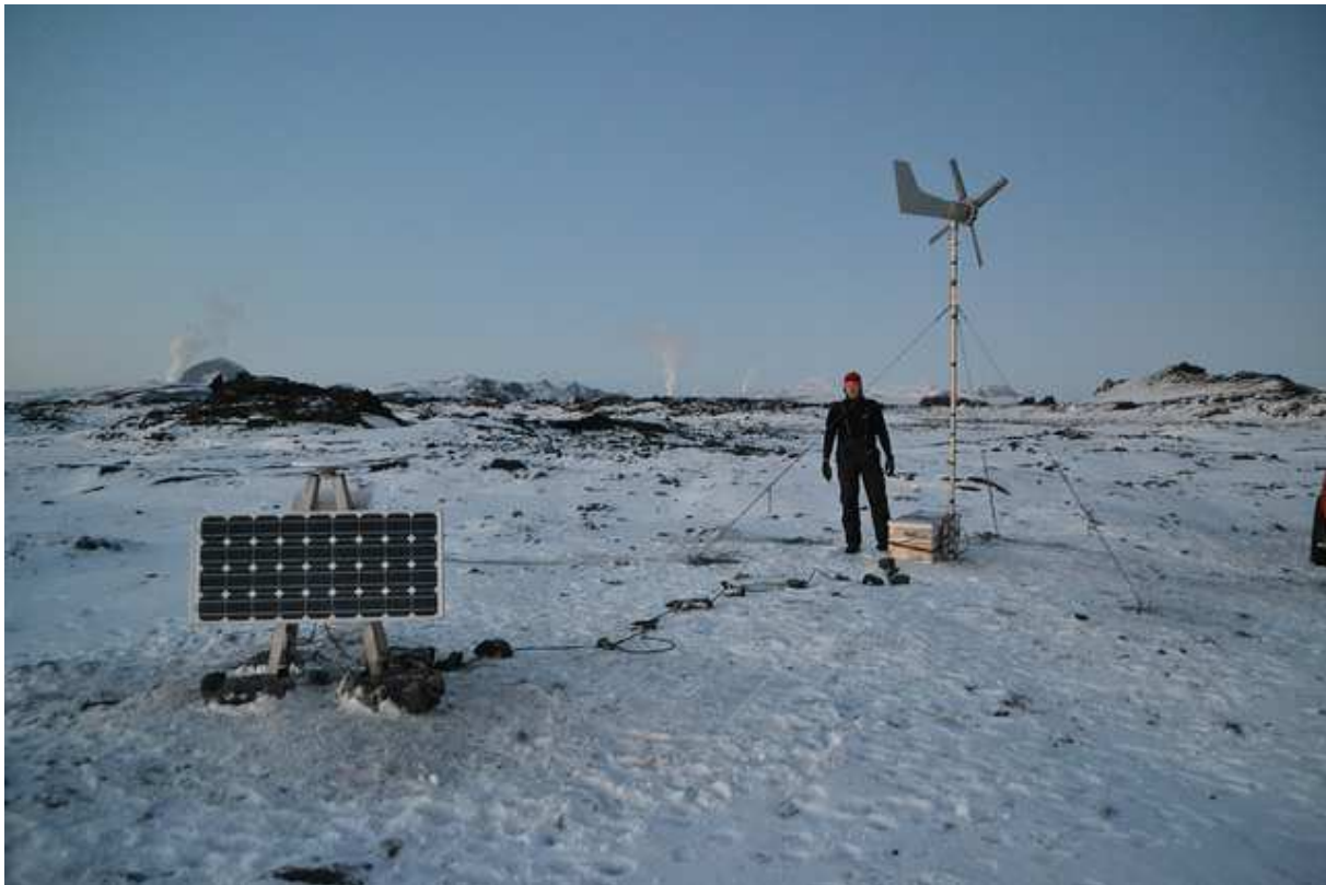
Figure 2.2: Picture of Bjarnarflag continuous GPS station (BJAC). It is supplied with both wind and solar energy.
