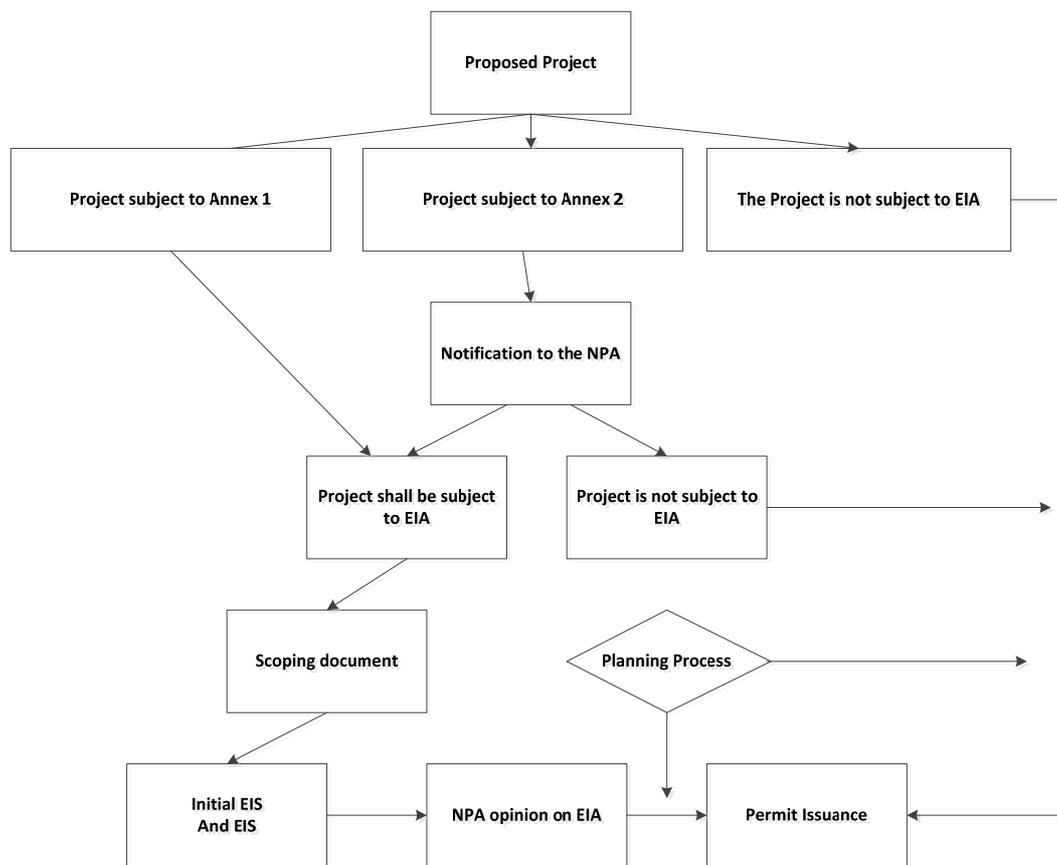
FIGURE 10: EIA project assessment for geothermal projects (Thóroddsson, 2012a)
