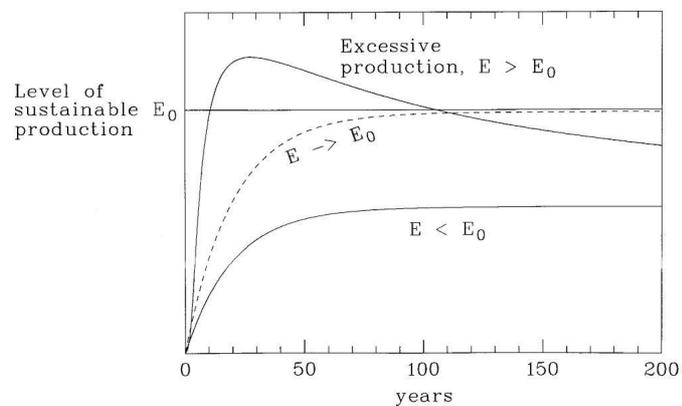
FIGURE 5: Sustainable production from a geothermal system (Axelsson et al., 2001)
