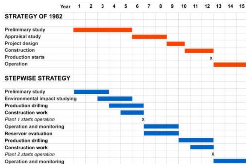
FIGURE 8: General plan and stepwise strategy for geothermal power plants (Steingrímsson, 2009)
