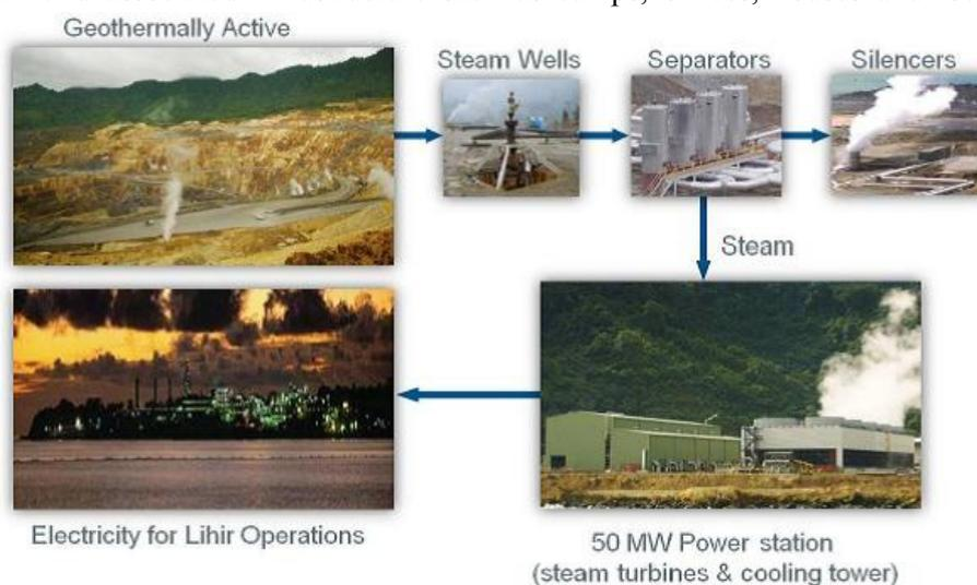
FIGURE 16: Lihir geothermal generation – how geothermal energy has been utilised in Lihir (Newcrest, 2012)
