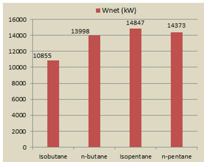
FIGURE 20: Net optimum output of the plant
