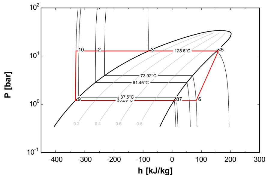
FIGURE 10: P-h diagram for model binary cycle
