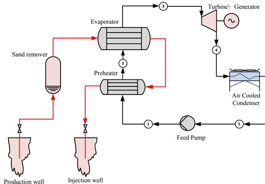
FIGURE 7: Schematic diagram of a basic binary cycle
