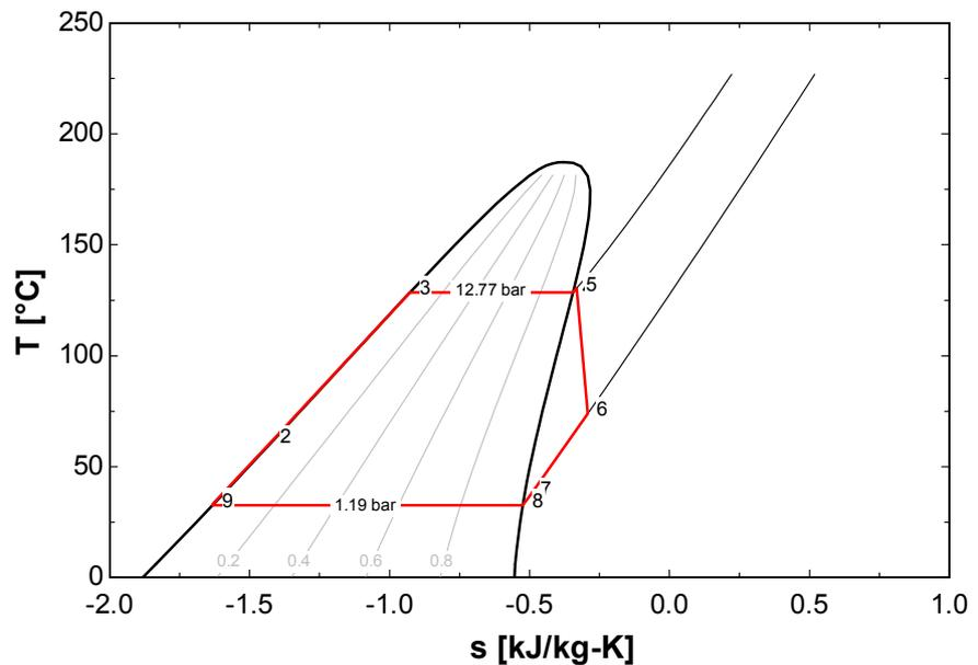
FIGURE 9: T-S diagram for model binary cycle
