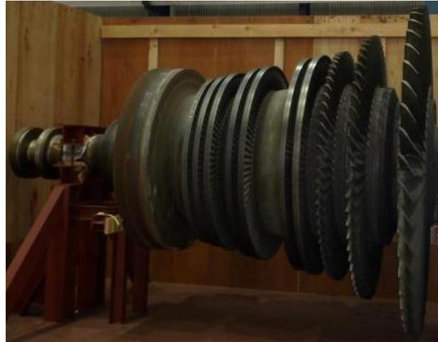
FIGURE 4: Steam turbine rotor
