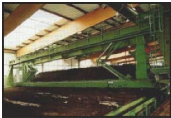
Mynd 2.1-16. Beddavinnsla innanhúss í Essenheim í Þýskalandi, (úr „Biological Treatment of Domestic Waste in Closed Plants in Europa - Plant Visti Reports“, RVF Report 98:8)
