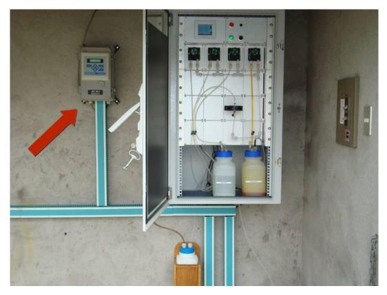
FIGURE 14: pH instrument for continuously record pH values. Photo by P. Moya
