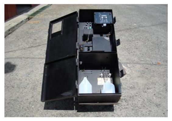
FIGURE 5b: Continuous flow analyzer from Rosemount Analytical Inc. Photo by P. Moya
