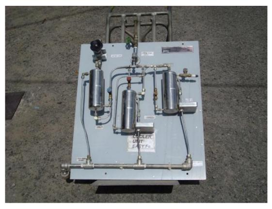
FIGURE 6: System to process the brine sample. Photo by P. Moya
