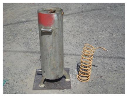
FIGURE 7: Spiral-type heat exchanger. Photo by P. Moya
