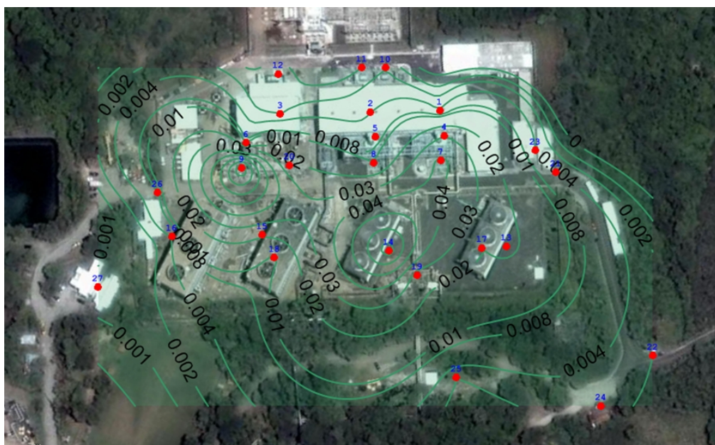
FIGURE 4: H 2 S concentration (ppm) in the air at the Berlín geothermal power plant in 2009
