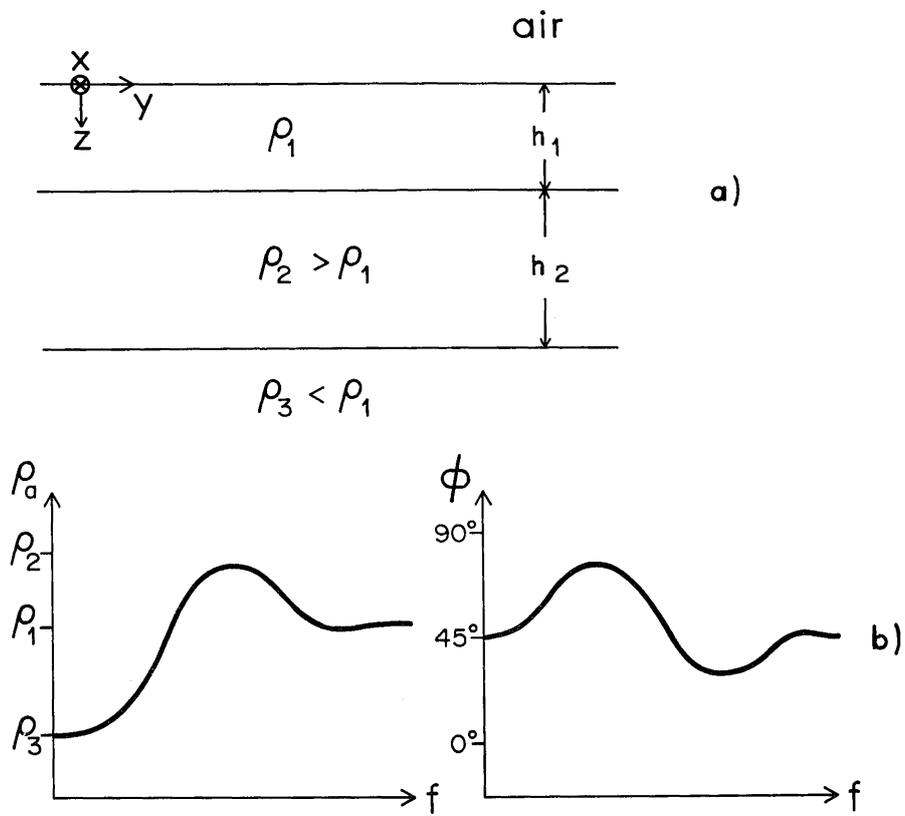
Figure 4: 1D MT apparent resistivity and phase.
