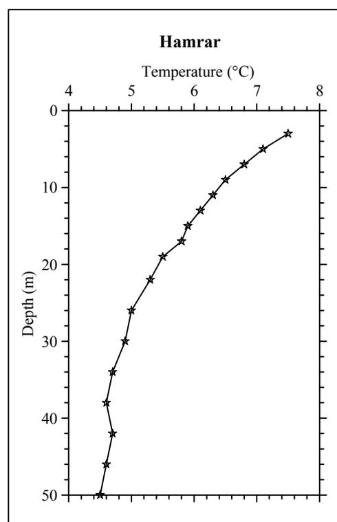
FIGURE 5: Temperature log in the KL well near Hamrar farm, from Oct. 5, 2004; note the reverse gradient
