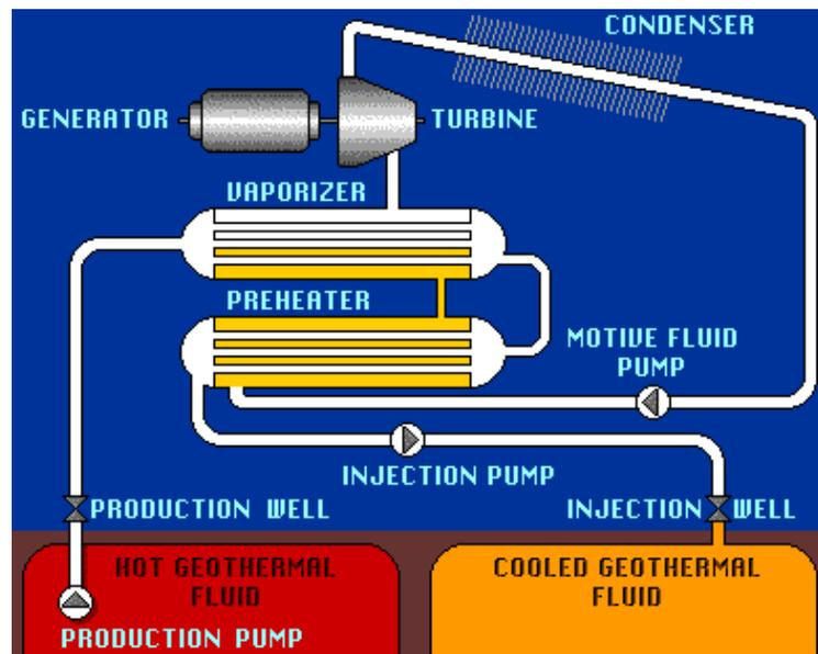
FIGURE 12: ORMAT energy converter (OEC)
