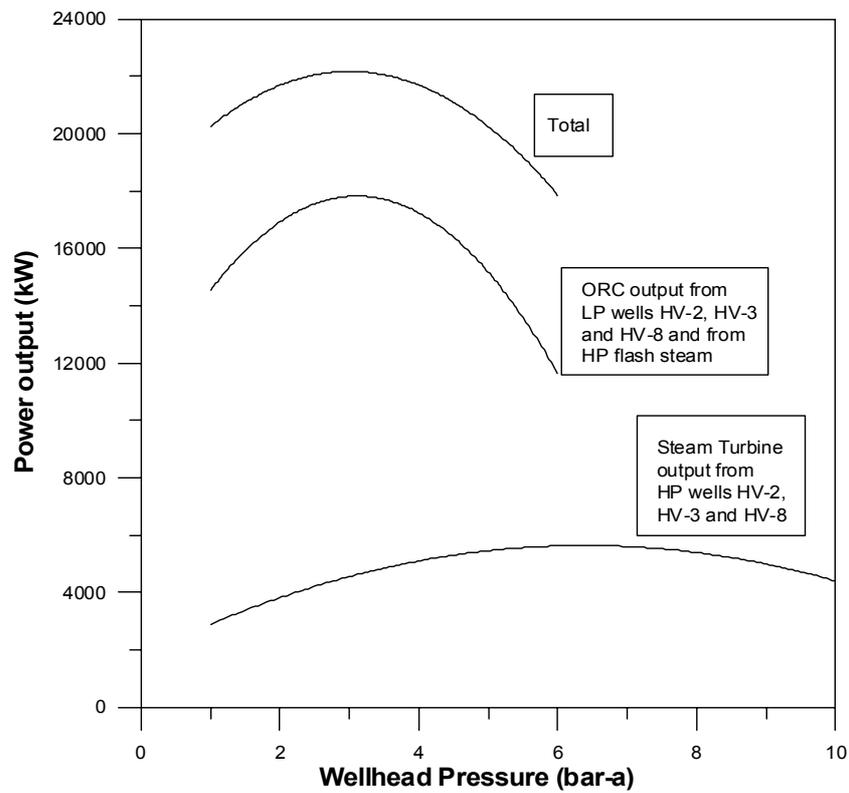
FIGURE 16: Optimum power output and well head pressure
