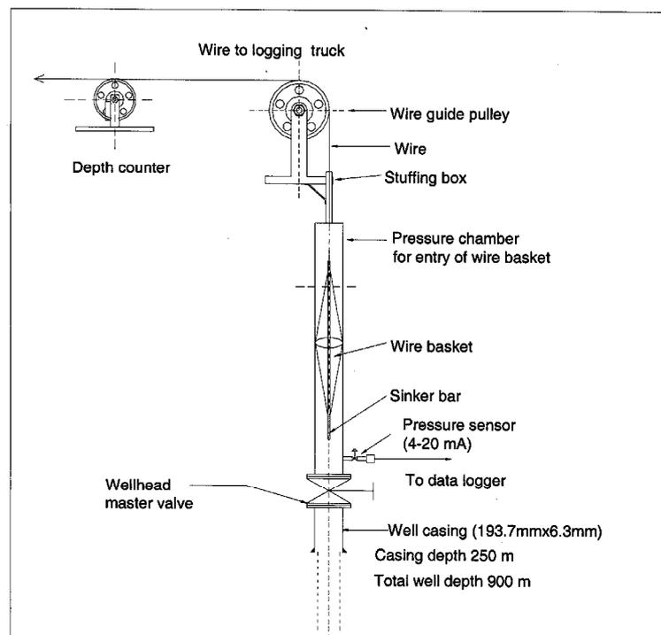
FIGURE 3: Sketch of a wire basket for scaling measurement in a production well
