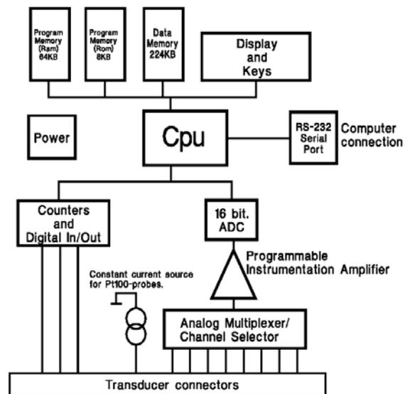
FIGURE 8: Photo and functional block diagram of the INTAB 2100-logger
