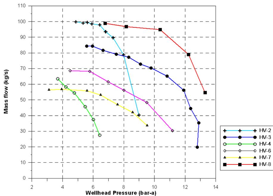
FIGURE 14: The flow characteristics of the Ölfusdalur wells
