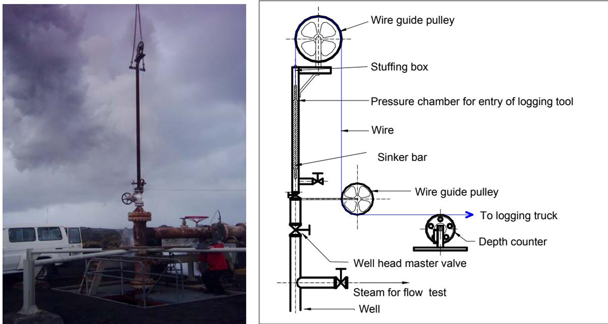
FIGURE 6: Wellhead for logging tools for temperature and pressure while the well is flowing.
