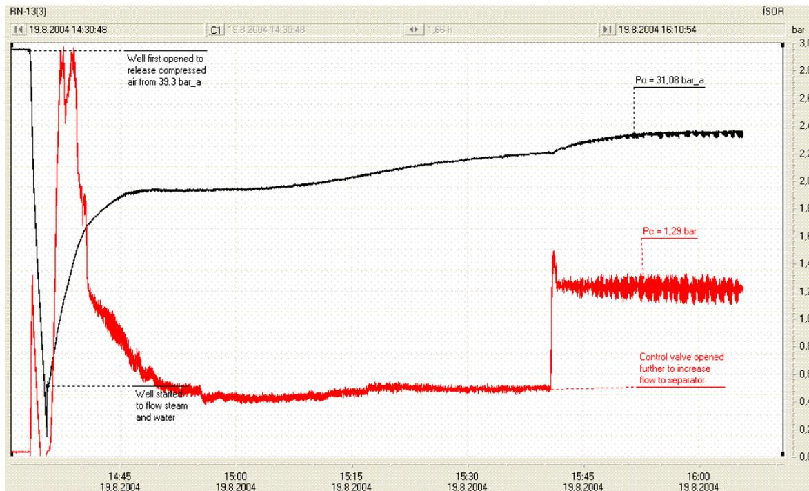
FIGURE 9: Data taken for two hours after initiating of well no. RN-13, Reykjanes, Iceland
