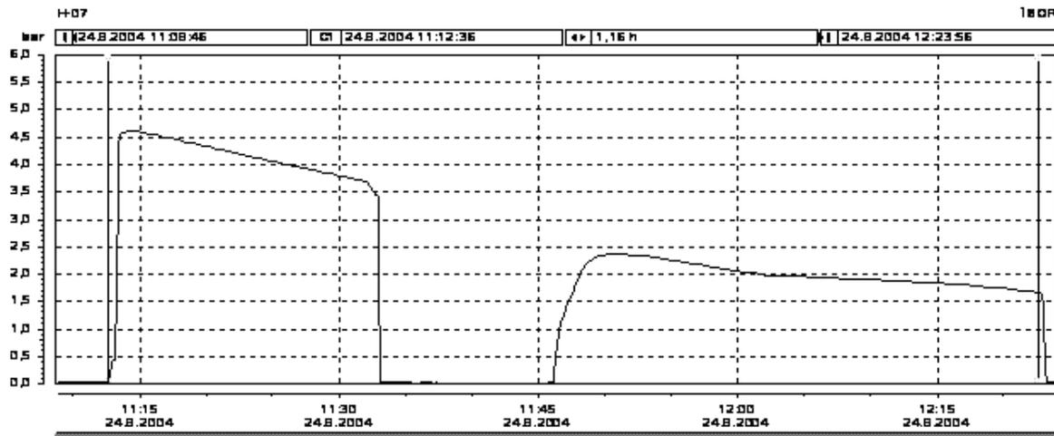
FIGURE 4: Wellhead pressure data taken when scaling measurement was done at well no. HE-07, Hveragerði, S-Iceland; the data was taken for 76 minutes. The decline in pressure is due to a slight leak on the stuffing box
