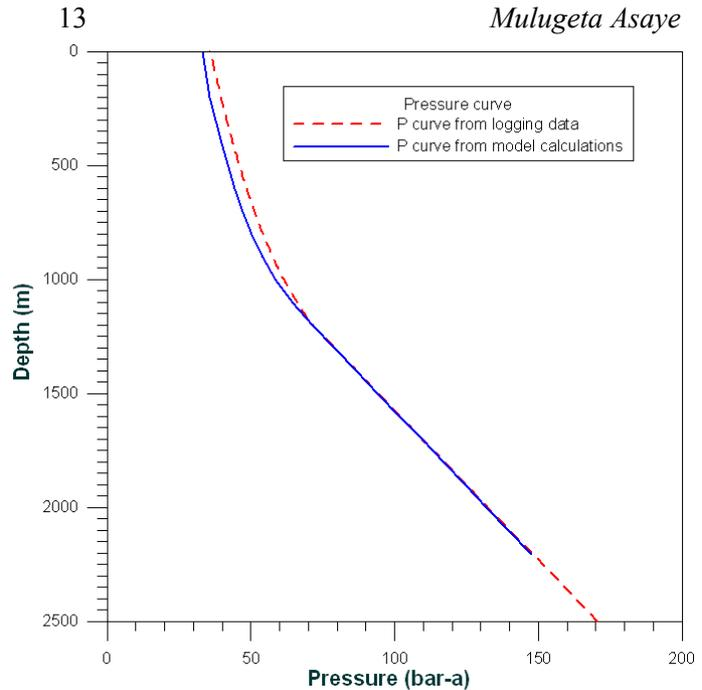
FIGURE 7: Pressure profile vs. depth in a 290°C flowing well
