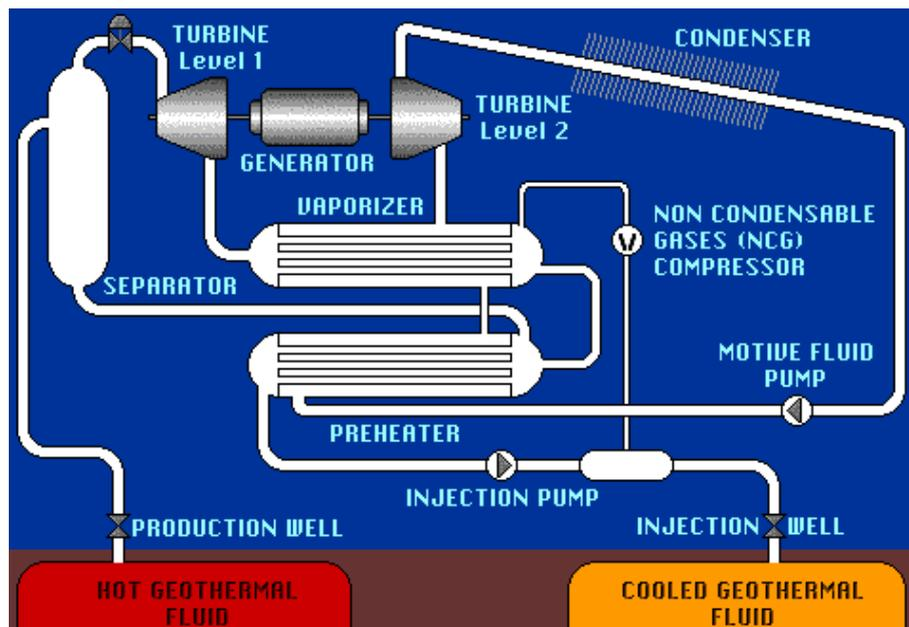
FIGURE 13: ORMAT geothermal combined cycle unit (GCCU)
