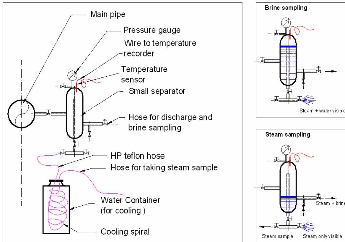
FIGURE 11: A portable separator to collect steam and brine samples
