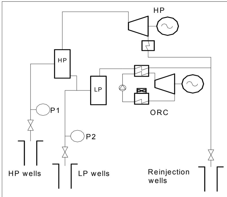
FIGURE 15: Diagram of power generation in high-pressure and ORC turbines from low-pressure and high-pressure wells on the basis of model calculations
