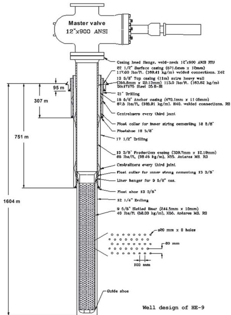
FIGURE 6: Schematic well design of well HE-9 (Thórhallsson, 2003)
