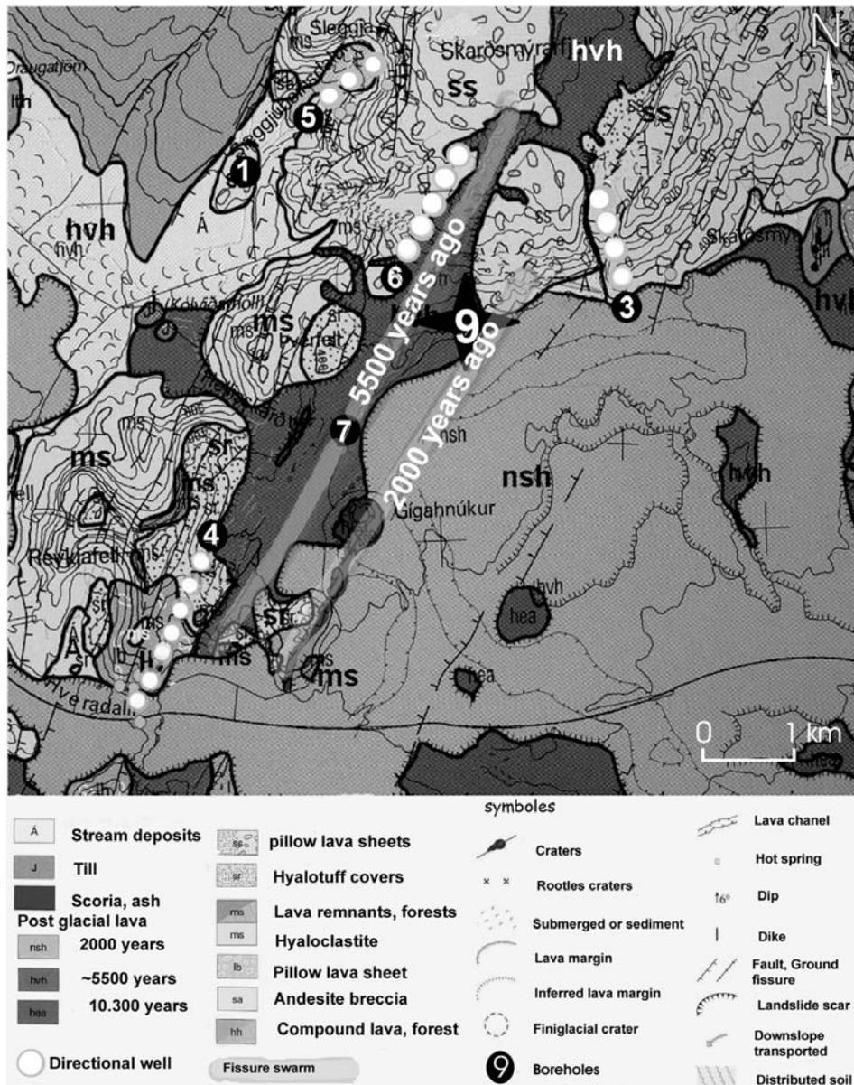
FIGURE 4: Geological map of Hellisheidi geothermal field showing boreholes (modified after Saemundsson, 1995)
