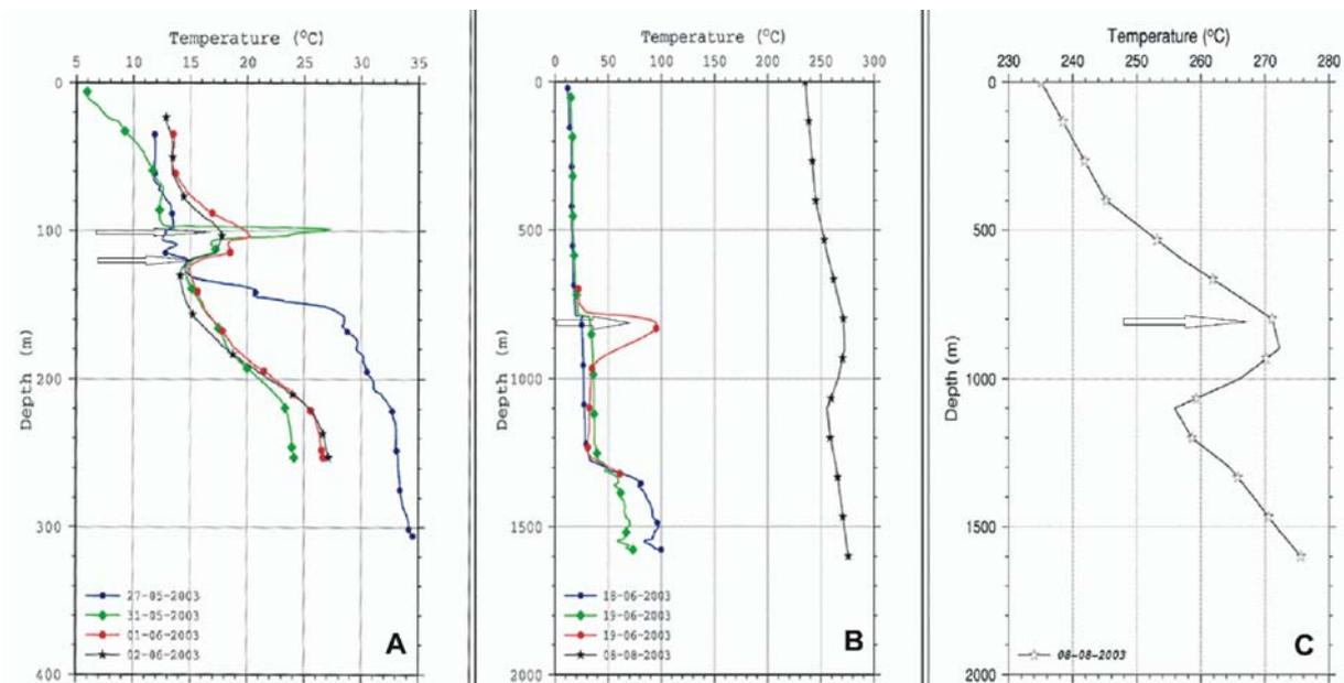
FIGURE 12: Temperature logs indicating 3 possible aquifers in the well HE-9
