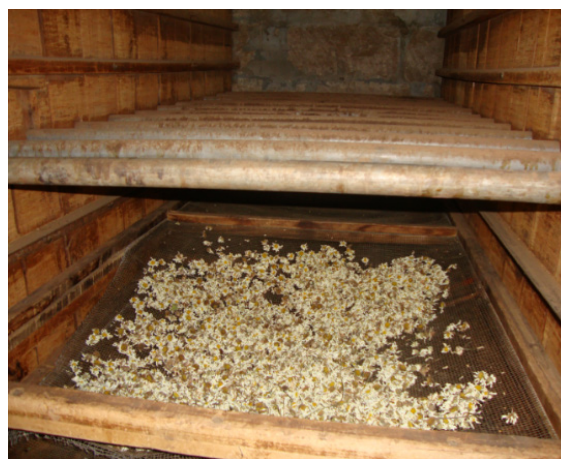
FIGURE 22: Pyrethrum drying using geothermal heat in Eburru, Kenya
