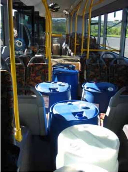
Figure 35 Barrels full of water and sand can substitute passenger load on public buses
