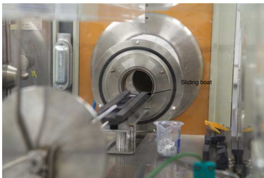
Figure 3.4: Inside the glovebox. In the process, the graphite boat is placed on top of the graphite slider.
