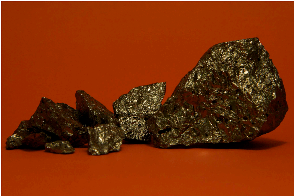
Figure 2.5: The MG-Si rocks that were used as the starting materials for the substrates. In a traditional process, they are melted and re-crystallized to produce solar-grade silicon.
