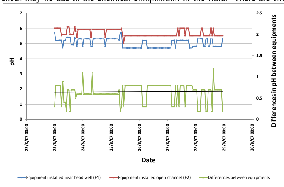
FIGURE 13: pH data, the data from the open channel are always higher than those from the samples taken near the head; with only minor variations in the difference (green line), being close to the value 0.70
