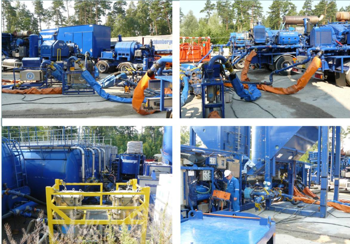
FIGURE 22: Instrumentations at the Groß Schönebeck drill site during the stimulation treatments in GrSk 4/05. From the upper left to the lower right photo: (1) equipment to connect the pipe at the surface, (2) pumping aggregates to pump 150 l/s against 600 bar, (3) tank volume of more than 1,000 m<sup>3</sup>, and (4) container to store proppants for the hydraulic proppant frac
