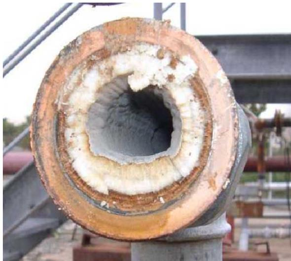
FIGURE 29: Carbonat scaling after some time of utilisation at a geothermal site
