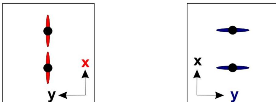
FIGURE 21: Conceptual arrangements of bottom hole positions in relation to fracture propagations. Left is a serial arrangement with fractures along the connection line of both wells and right, a parallel arrangement. Both wells in a thermal loop have in the serial arrangement dominantly artificial pathways whereas in the parallel arrangement, the fluid flow has to pass the rock on natural pathways
