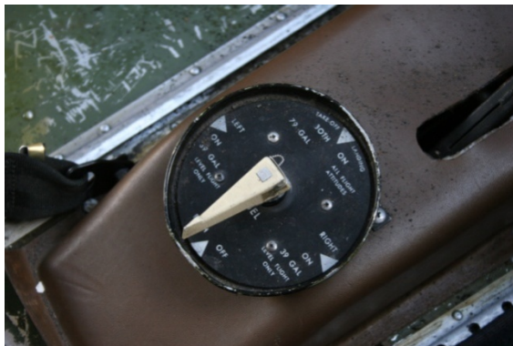
Figure 4: Fuel selector valve
