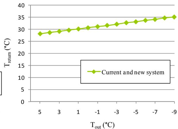
FIGURE 12: Change of return temperature according to outdoor temperature, for the floor heating system
