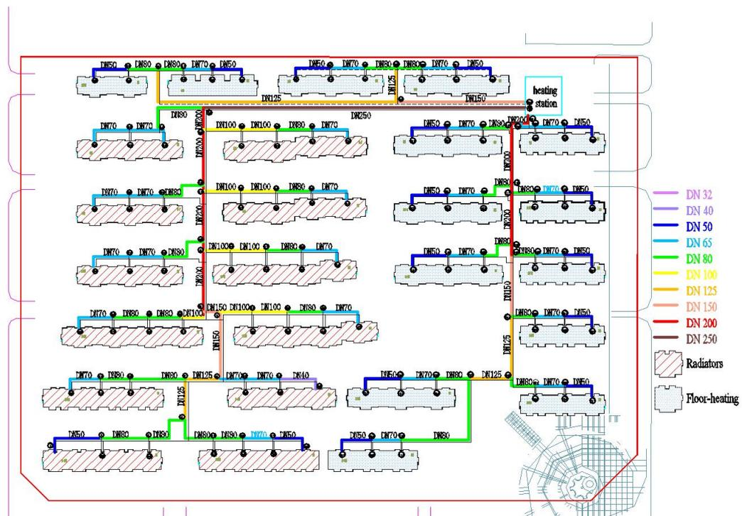
FIGURE 7: Distribution system layout for the current heating system
