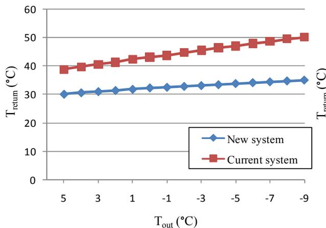
FIGURE 11: Change of return temperature according to outdoor temperature in the radiator systems
