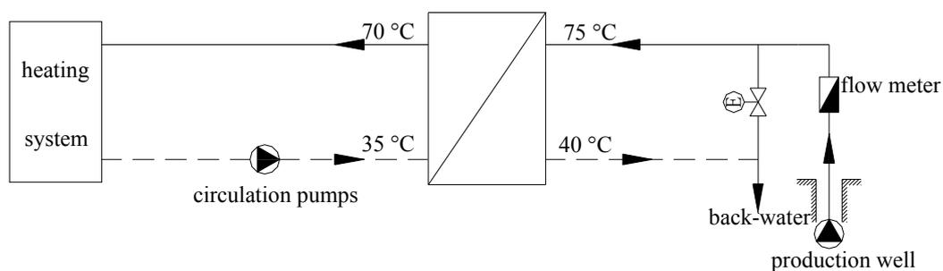
FIGURE 5: Flow chart of the new heating system
