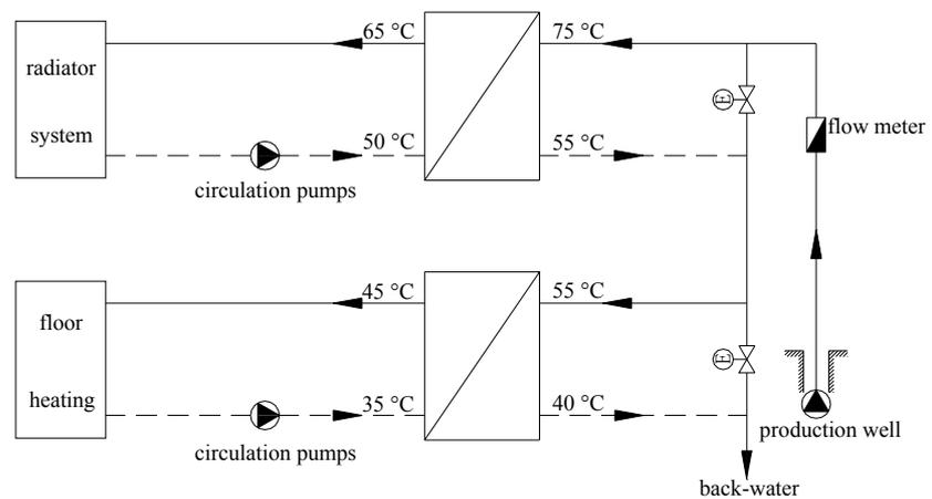
FIGURE 4: Flow chart of current heating system
