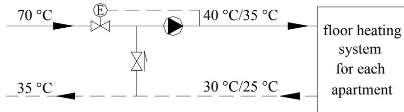
FIGURE 6: Flow chart of the new substations
