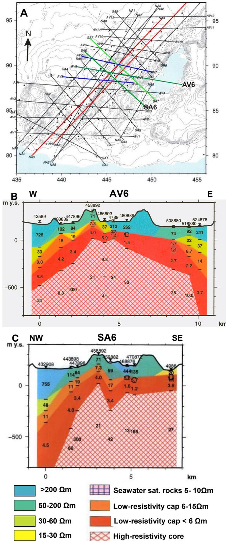
FIGURE 7: Resistivity measurements in Trölladyngja-Sog area, a) Location map showing the distribution of the TEM soundings; b) Cross-section AV6, with a W-E trend through the Trölladyngja-Sog area; and c) Cross-section SA6 trending NW-SE; the cross-section show resistivity structures associated with the geothermal upflow
