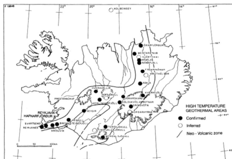
FIGURE 3: High-temperature geothermal areas in Iceland (Ármannsson et al., 1994)
