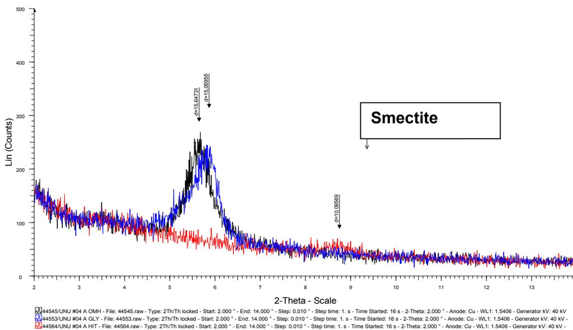
FIGURE 3: XRD analysis of sample AMD.029
