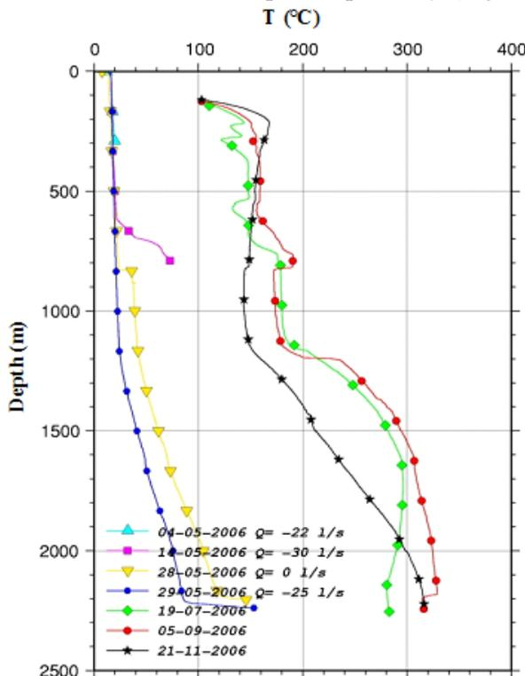
FIGURE 6: Temperature profiles of well TR-02 in Trölladyngja area (ISOR-database)
