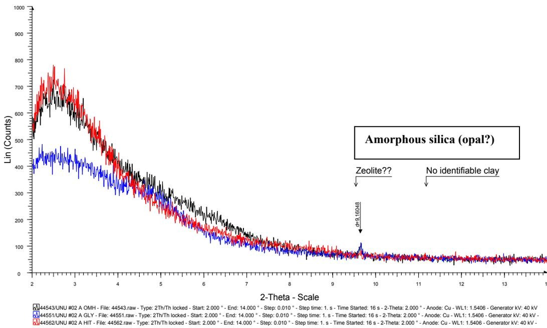
FIGURE 6: XRD analysis of sample AMD.031
