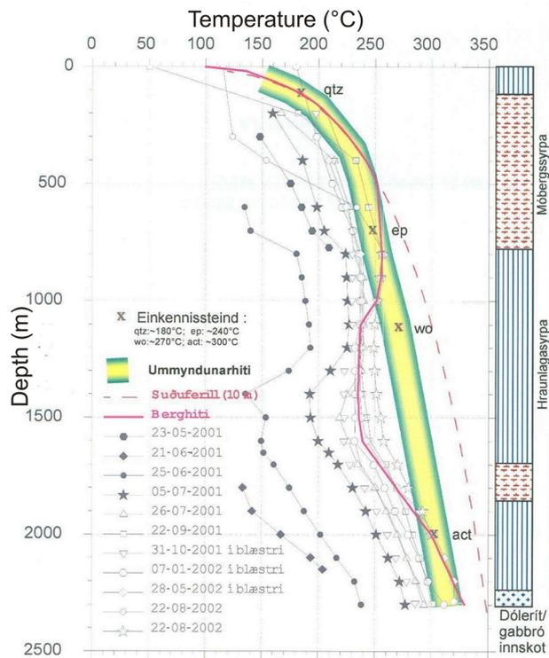
FIGURE 5: Temperature profiles of well TR-01 in Trölladyngja area (Fridleifsson et. al., 2002)
