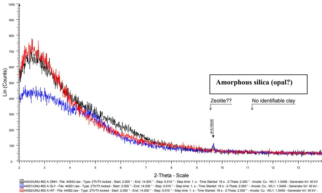
FIGURE 6: XRD analysis of sample AMD.031
