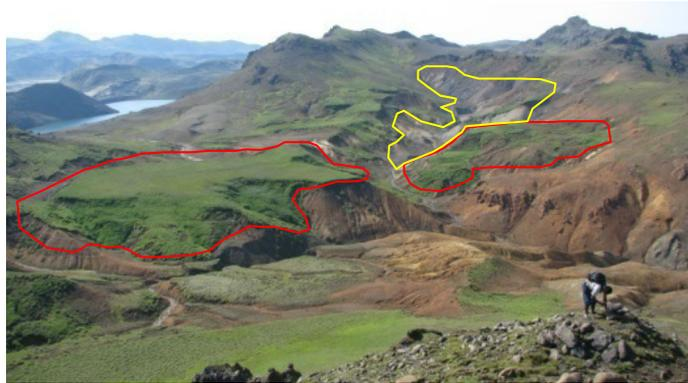
FIGURE 10: Holocene sediments (red polygons) and grayish to bluish alteration (yellow polygon) around the Sog valley
