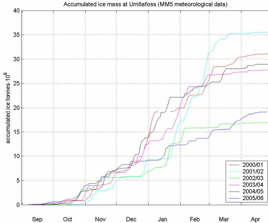
**Figure 6:** *Accumulated ice mass at Urriðafoss, according to calculations with meteorological data from MM5.*
