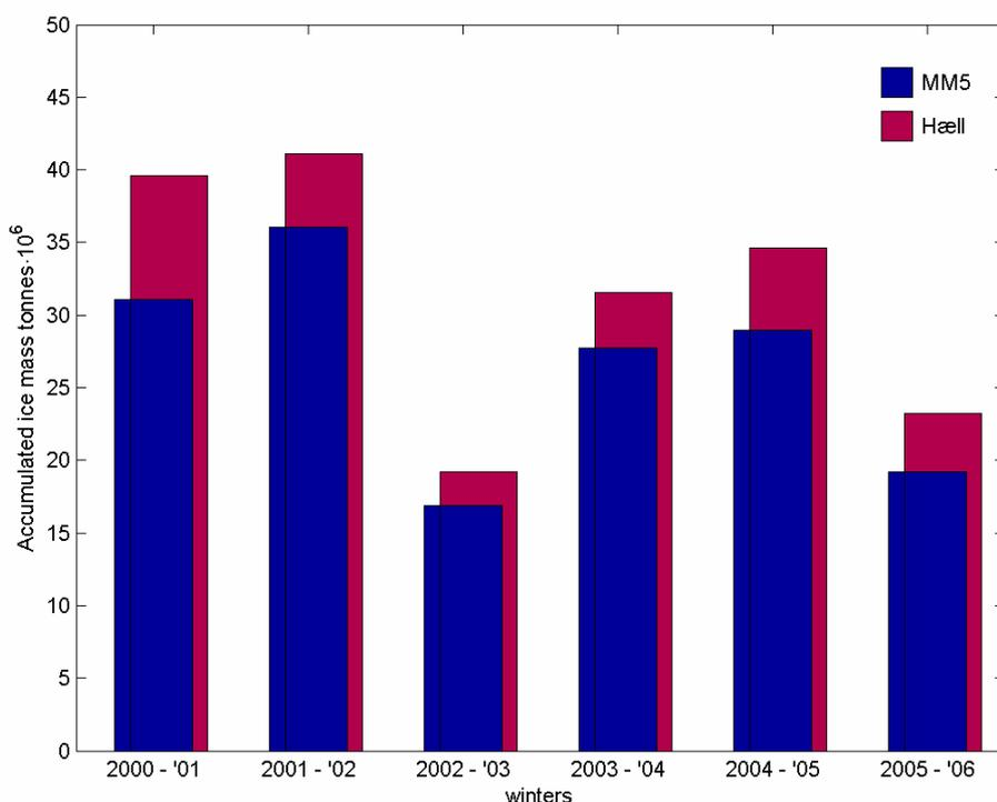
**Figure 7:** Comparison of accumulated ice mass at Urriðafoss, according to MM5 and Hæll calculations.
