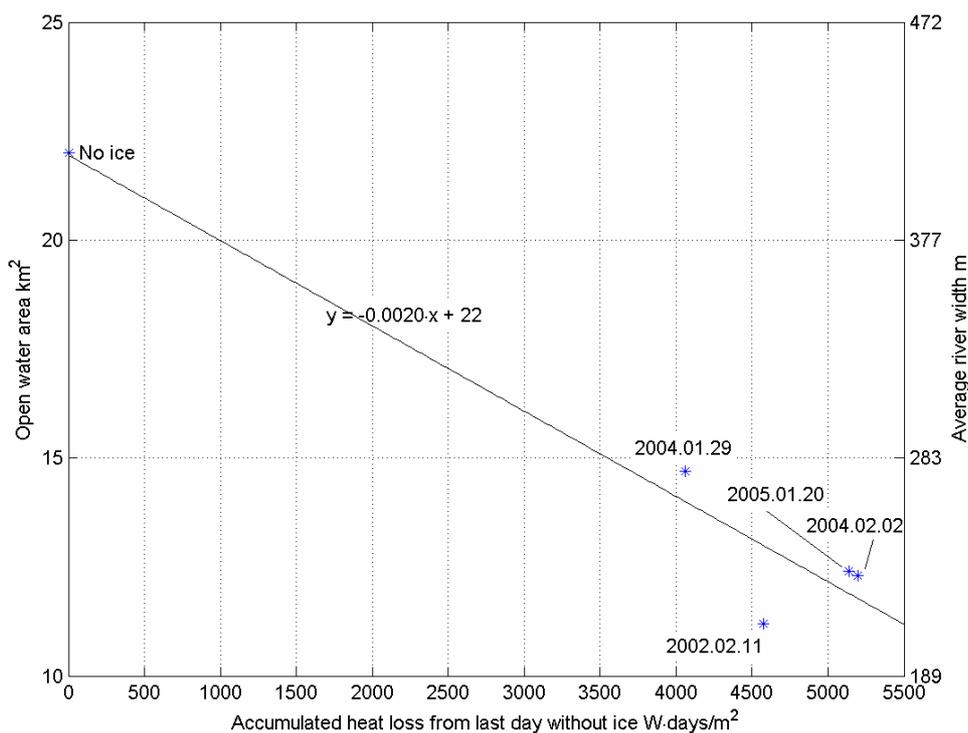
**Figure 2:** *Open water area and accumulated heat loss. Data from Helgason and Gröndal (2006) and Helgason (2002).*
