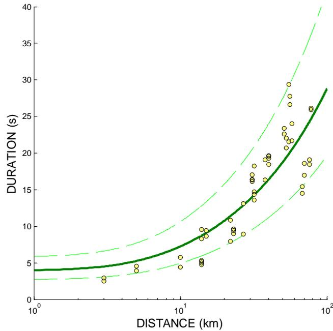
Figure 3 Relative significant duration of shallow strike-slip earthquakes. The duration values obtained for the June 2000 South Iceland Earthquakes compared to suggested duration model (solid line). The dashed lines represent the model  $\pm$  one standard deviation of full dataset.
