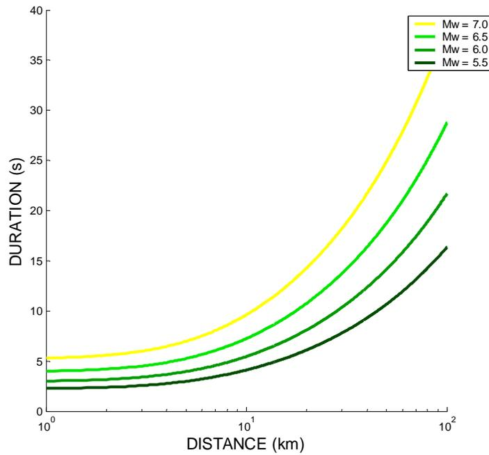
Figure 4 Relative significant duration of shallow strike-slip earthquakes with near vertical fault plane. Suggested model representing duration as a function of distance to surface trace of causative fault for different magnitude values.
