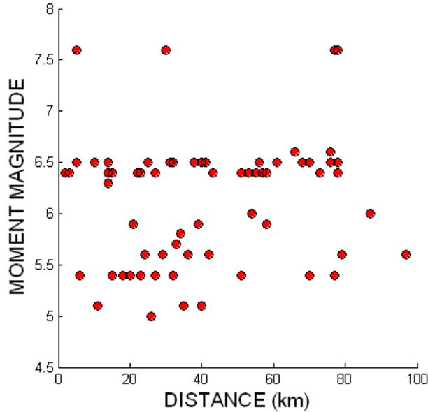
Figure 1 Distribution of the applied data in terms of moment magnitude and source distance. The data set shown contains 71 tri-axial strong-motion records recorded at rock sites in 13 shallow strike-slip earthquakes.
