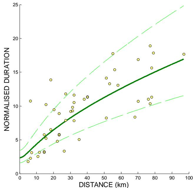
Figure 2 Relative significant duration of shallow strike-slip earthquakes. The solid line is the suggested model obtained by regression analysis and the circles are data from the applied dataset. The dashed lines represents gives the model  $\pm$  one standard deviation.
