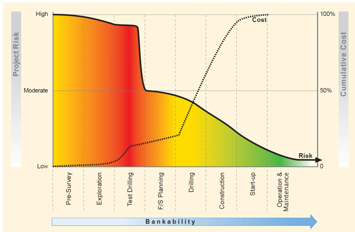
FIGURE 1: Project cost and risk profile at various stages of development – Electricity project (Gehring and Loksha, 2012)
