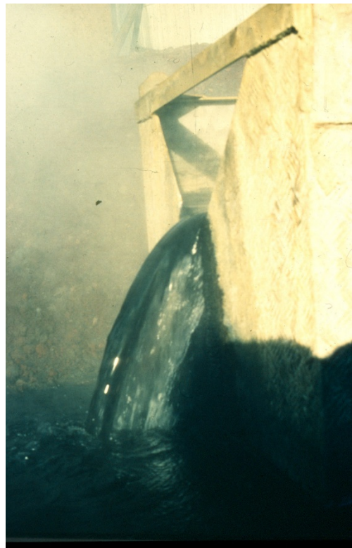
FIGURE 6: Iron sulphide and silicate deposits in flow from a Krafla well
