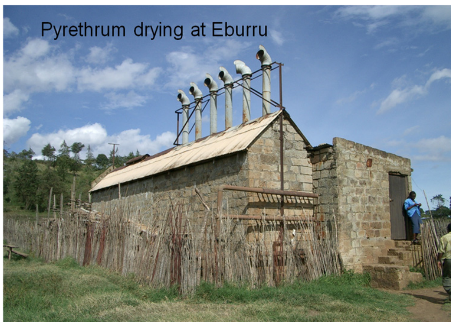
FIGURE 7: Geothermal energy being used by the local community at Eburru for pyrethrum drying
