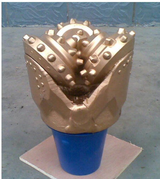
FIGURE 3: A typical roller cone bit used in Menengai
