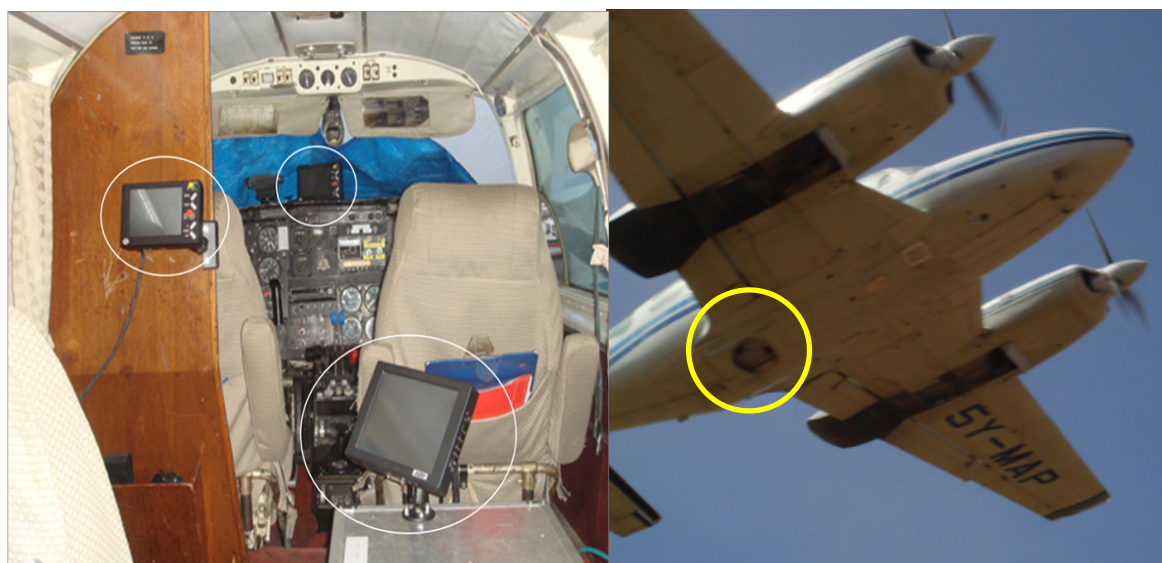
FIGURE 3: Touch screen monitors for operating the Thermal camera and the camera hatch as seen from below the aeroplane
