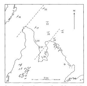
Fig. 6. The cone-sheet-complex with mean strike and dip symbols. The central part of the plagioclase-augite-porphyritic dyke-swarm (p. 25) lies between the broken lines.
