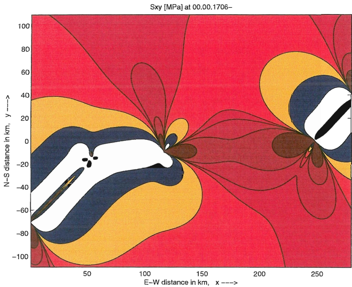
Figure 62. Shear stress field in the South Iceland seismic zone and its surroundings as assumed in 1706 ("short rupture model"). — The values of the isolines as in Figure 61 apply.
