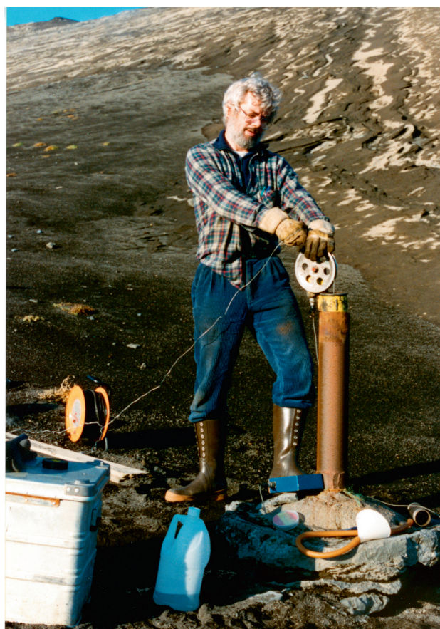
Fig. 2. Water sample collected downhole from drill hole SE-1 at Austurbunki in 1990.
