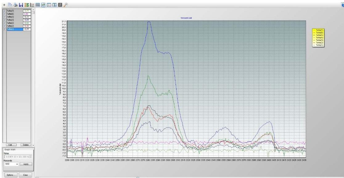
Figure 7. Test data from a pull of a 3 ton vehicle. The figure show data from 7 strain gauges.
