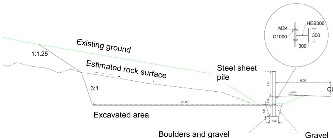
Figure 4. Typical cross section from the IRCA bid documents.
