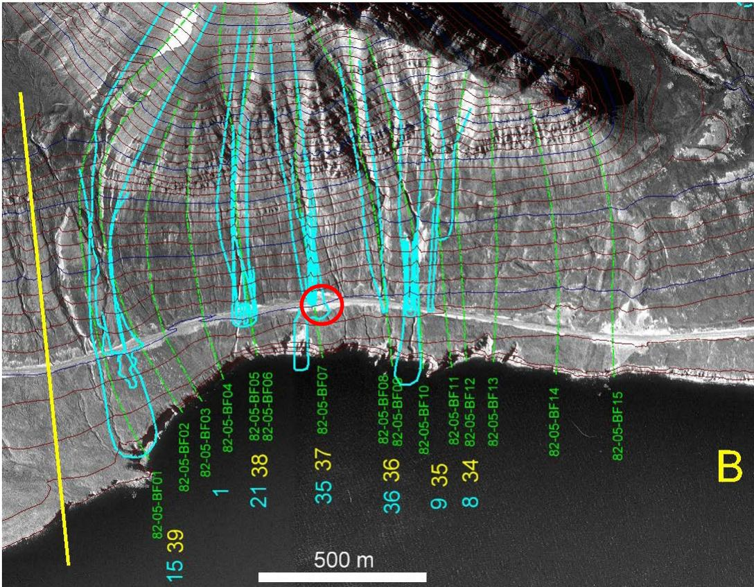
Figure 2. Avalanche paths and registered avalanches (cyan lines) north of Sauðanes. Red circle denotes the test site. Yellow numbers show the IRCA avalanche path numbering system. Cyan numbers show number of avalanches for the period 1974-2000. Green numbers and paths show paths used in [1]. Aerial photo: LMI.
