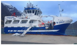
21m gillnet vessel with 270kWh battery capacity. 2X 850 kW generators and 2X 325kW electric propulsion
