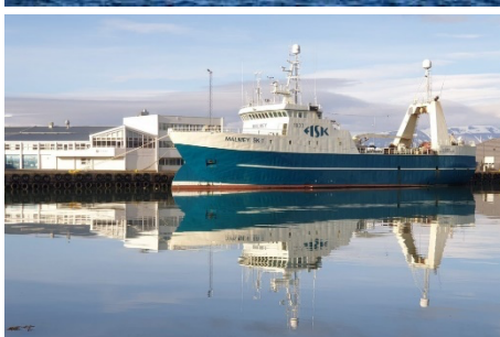
Trawler 4: Málmey SK 1 Built in 1987 Length: 56,50 m. Width: 12,60 m. GT: 1.470 t. Hp: 2.991 Home port: Sauðárkrókur, Iceland Owner: FISK-seafood ehf
