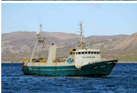
Trawler 3: Klakkur SK 5 Built in 1977 Length: 51,83 m. Width: 10,76 m. GT: 745 t. Hp: 2.200 Home port: Sauðárkrókur, Iceland Owner: FISK-seafood ehf
