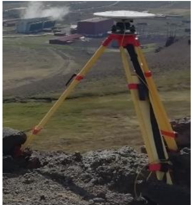
Figure 3. GNSS measurements. Left: a continuous GNSS site (KRAC), which collects data night and day for long times. Right: GNSS temporary set-up of equipment during campaign measurements (shorter time, typically several days, for each single GNSS site).
