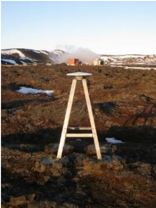
Figure 3. GNSS measurements. Left: a continuous GNSS site (KRAC), which collects data night and day for long times. Right: GNSS temporary set-up of equipment during campaign measurements (shorter time, typically several days, for each single GNSS site).
