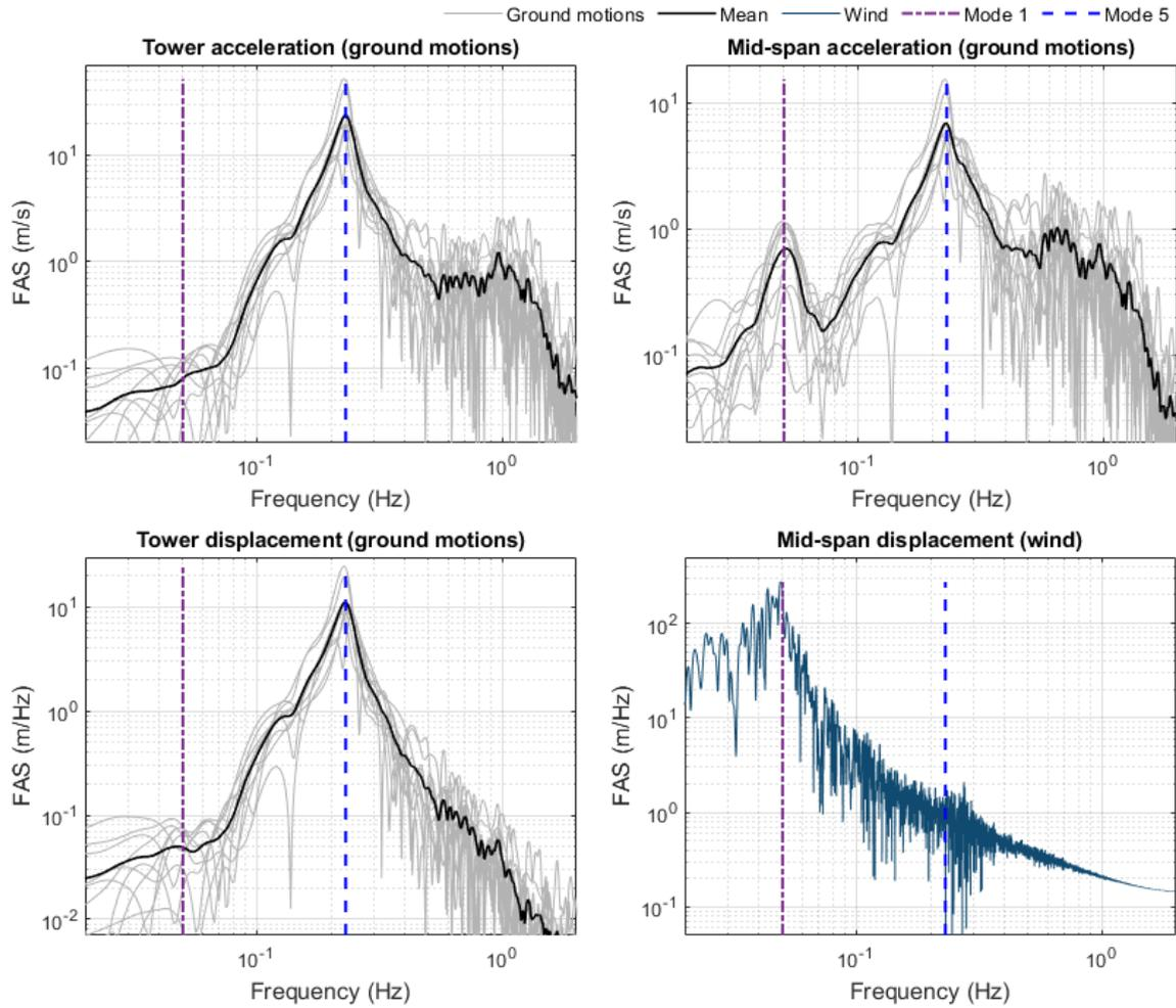
Figure 10. FSA of tower and mid-span acceleration and displacement response in transverse direction due to wind-induced force and ground motions.
