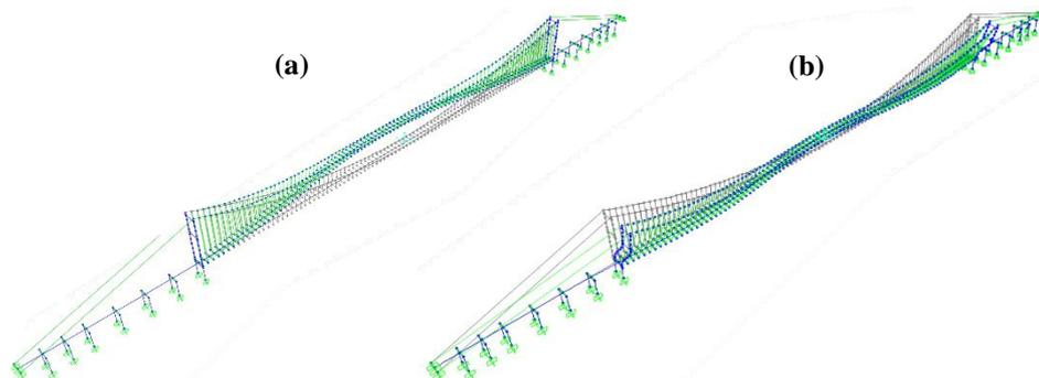
Figure 4. Mode shapes of the RSB, (a) Mode-1, the first horizontal symmetric mode, (b) Mode-5, the first tower transverse mode,
