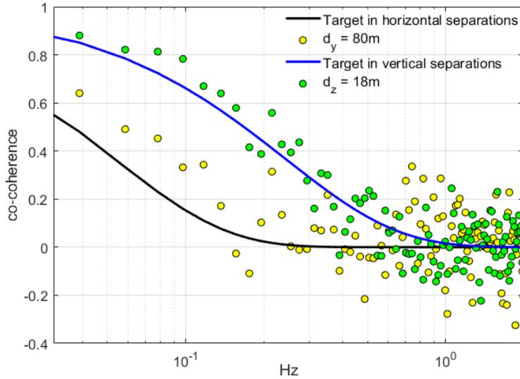
Figure 9, Co-Coherence of wind velocity in horizontal and vertical separations.
