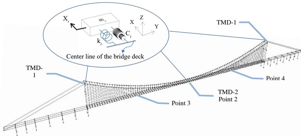
Figure 3. A FE model of the RSB showing the locations of the TMDs investigated in subsequent sections. The TMDs move only in the transverse direction of the bridge.
