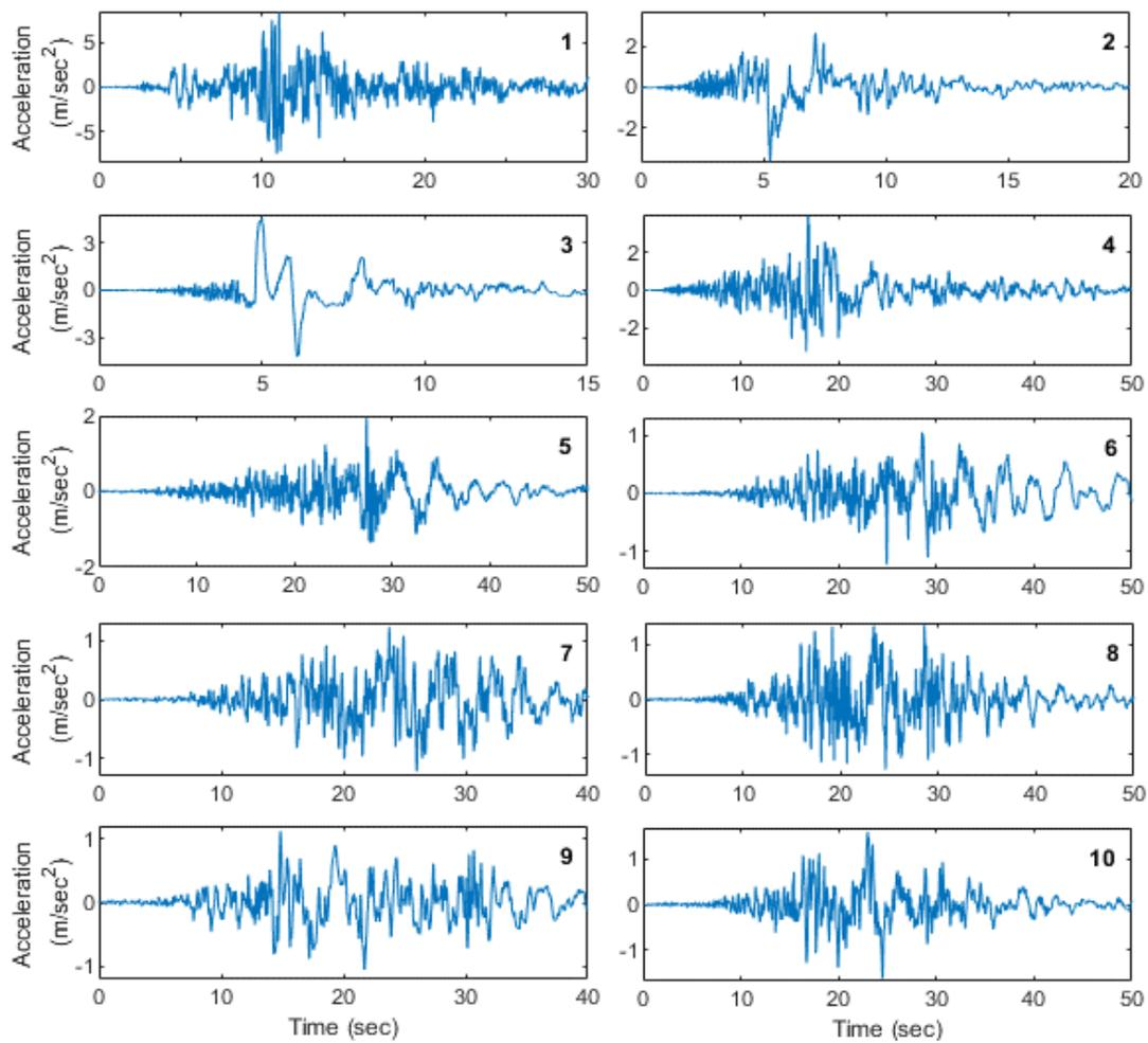
Figure 5. Time histories of the ground accelerations listed in Table 2.
