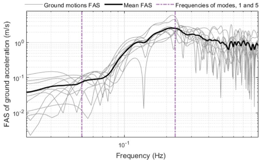
Figure 6. Fourier amplitude spectra (FAS) of the selected horizontal ground motion time series shown in Figure 5. The grey lines correspond to individual ground motions and the black line is the average FAS. The vertical lines correspond to the frequencies of the two modes listed in Table 1.
