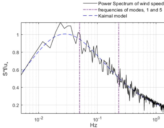
Figure 8. The power spectrum of wind speed at the centre of the deck (see Kaimal et al., 1972).
