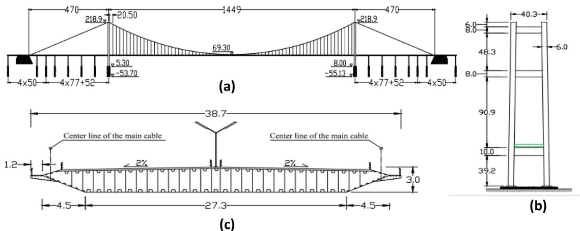
Figure 2. The RSB (a) elevation. (b) Geometry of the tower. (c) Cross-section girder. (Dimensions in m)
