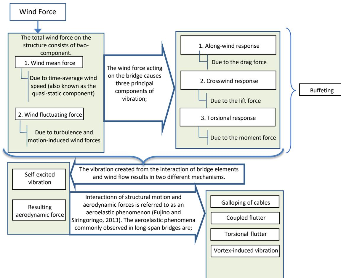
Figure 1 Wind-induced vibration mechanisms (based on Fujino and Siringoringo, 2013).
