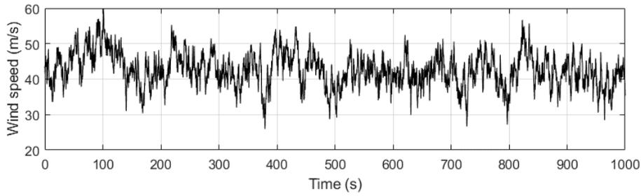
Figure 7. A sample time history of along-wind velocity at the centre of the deck.
