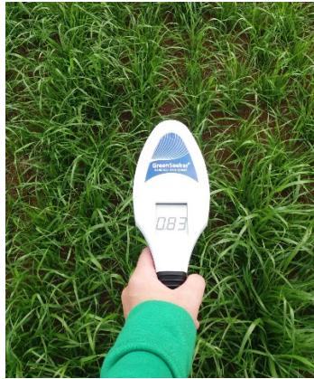
Figure 6: Exemplary measurement with the NDVI device (combination of two sensors). The NDVI value here is 0.83.
