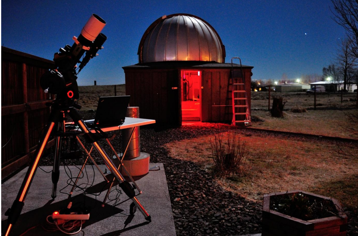
Mynd/Fig. 2. Tveir sjónaukar voru notaðir við athuganir haustið 2020. Skywatcher 80 mm linsusjónauka á Celestron AVX sjónaukastæði var stillt upp við skjólvegg en stærri sjónaukinn hýstur í stjörnustöðinni. – Two telescopes were used for observations in autumn 2020. A Skywatcher 80 mm refractor on a Celestron AVX German Equatorial mount was erected outside while the main telescope is housed in the observatory.
