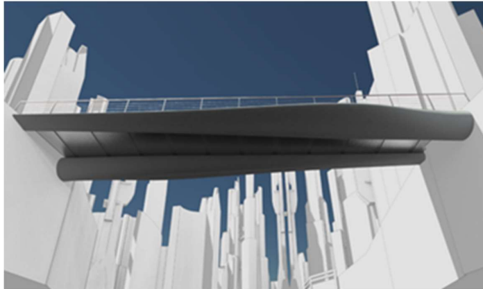
Figure 4 From a feasibility study on constructing bridges from wind turbine blades (Master Thesis at Delft University of Technology).
