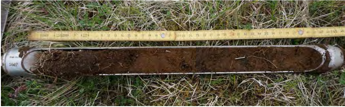
Figure 34: Layers in core 05_21. Cultural layers with charcoal (25-29 cm) and turf deposit with possible Hekla 1300 tephra (29-40 cm)
