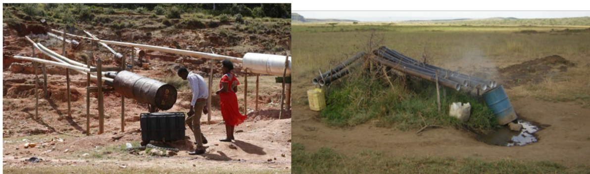
FIGURE 7: Domestic water harvesting from naturally occurring fumaroles at Eburru and Suswa
