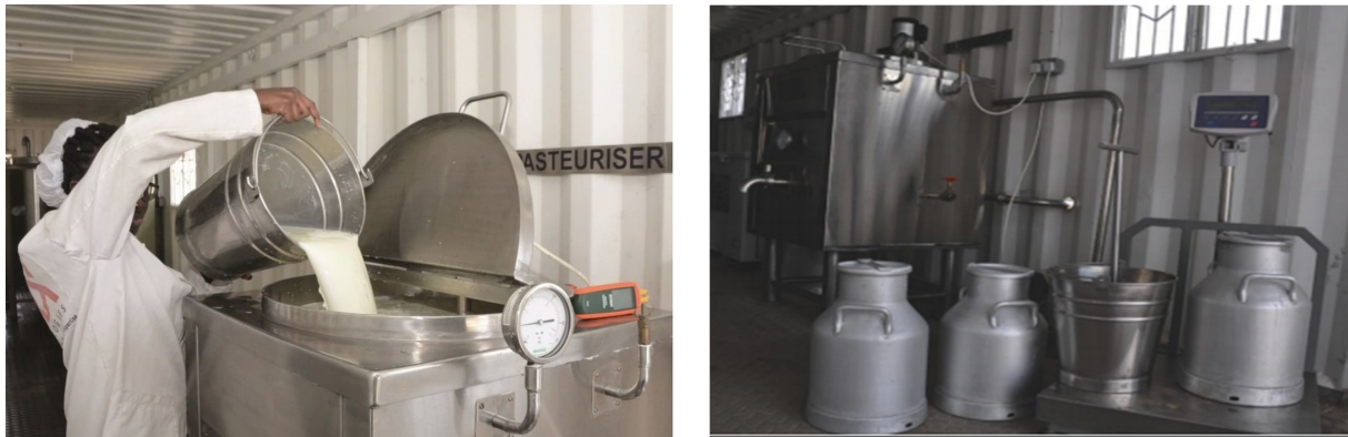
FIGURE 5: Geothermal-powered milk pasteurizer in Menengai
