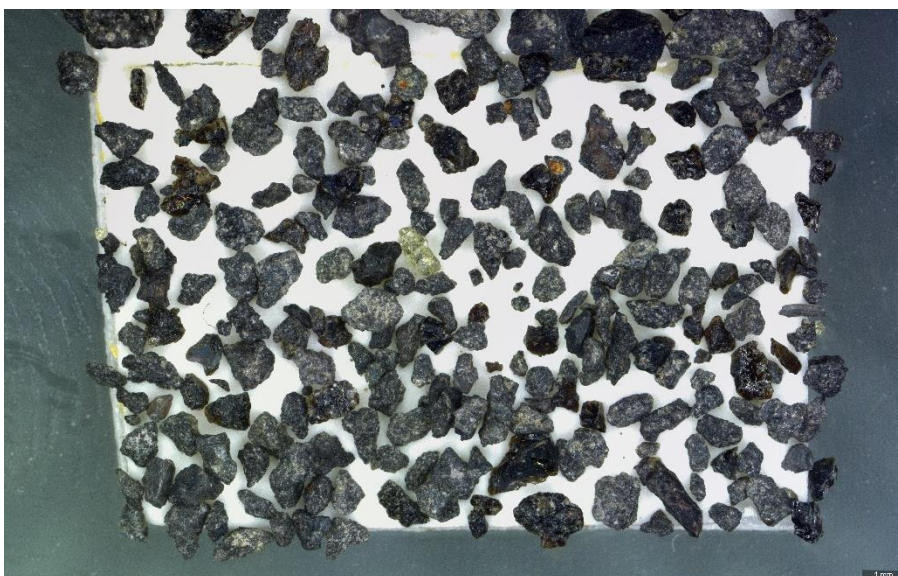
Figure 47 The <1 mm sample is similar to 1 mm but a little more glass. Only one loose PLAG.
