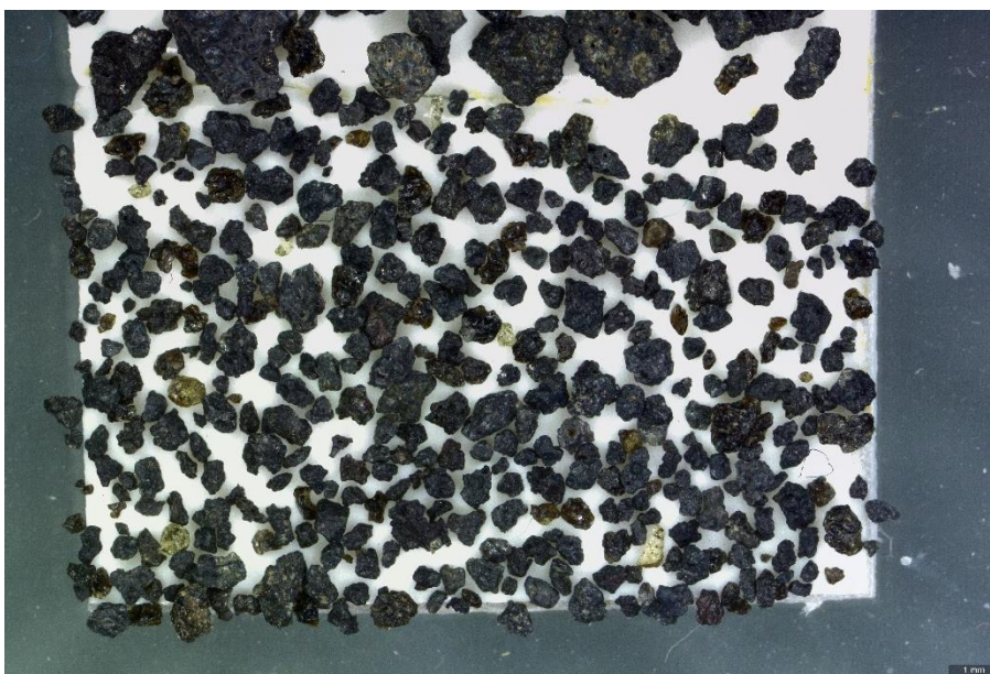
Figure 57 The <1 mm sample is the same as 1 mm. Loose OL and PLAG (<1%).
