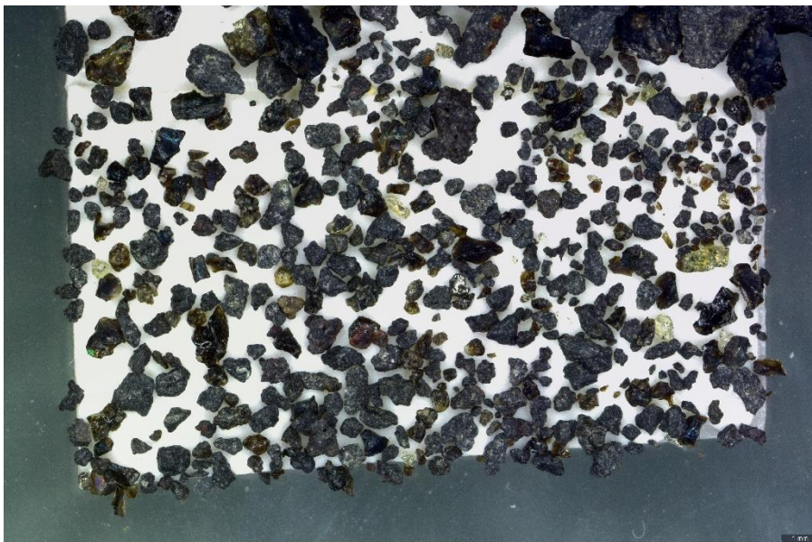
Figure 55 The <1 mm sample is the same as 1 mm. A little higher ratio of crystalline grains. Loose OL and PLAG crystals (~1%) No orange-red alteration.
