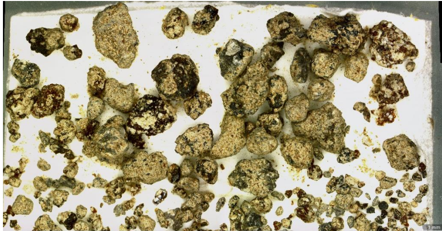
Figure 120 In the 1 mm sample there is altered coating (light yellow) on almost all grains, making distinction between them difficult. There are a few fully crystalline grains. There seem to be a few glass grains of varying crystallinity. Some red grains are present. Two crystalline grains have PLAG phenocrysts. Not many obvious phenocrysts are present overall, but the red grains contain white opaque minerals.
