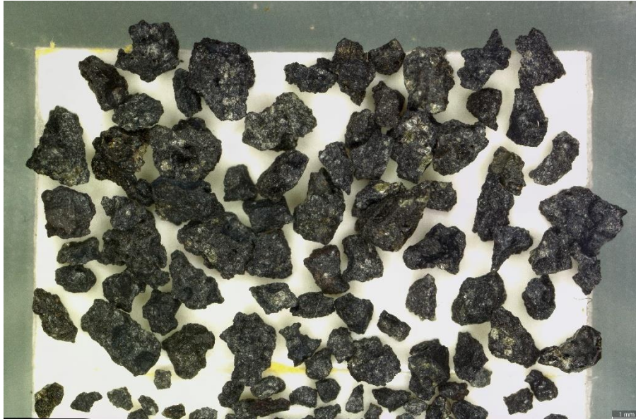
Figure 14 In the 1 mm sample there are only crystalline grains but darker than in BH4-4, not matte as in BH4-3. PLAG and OL common.
