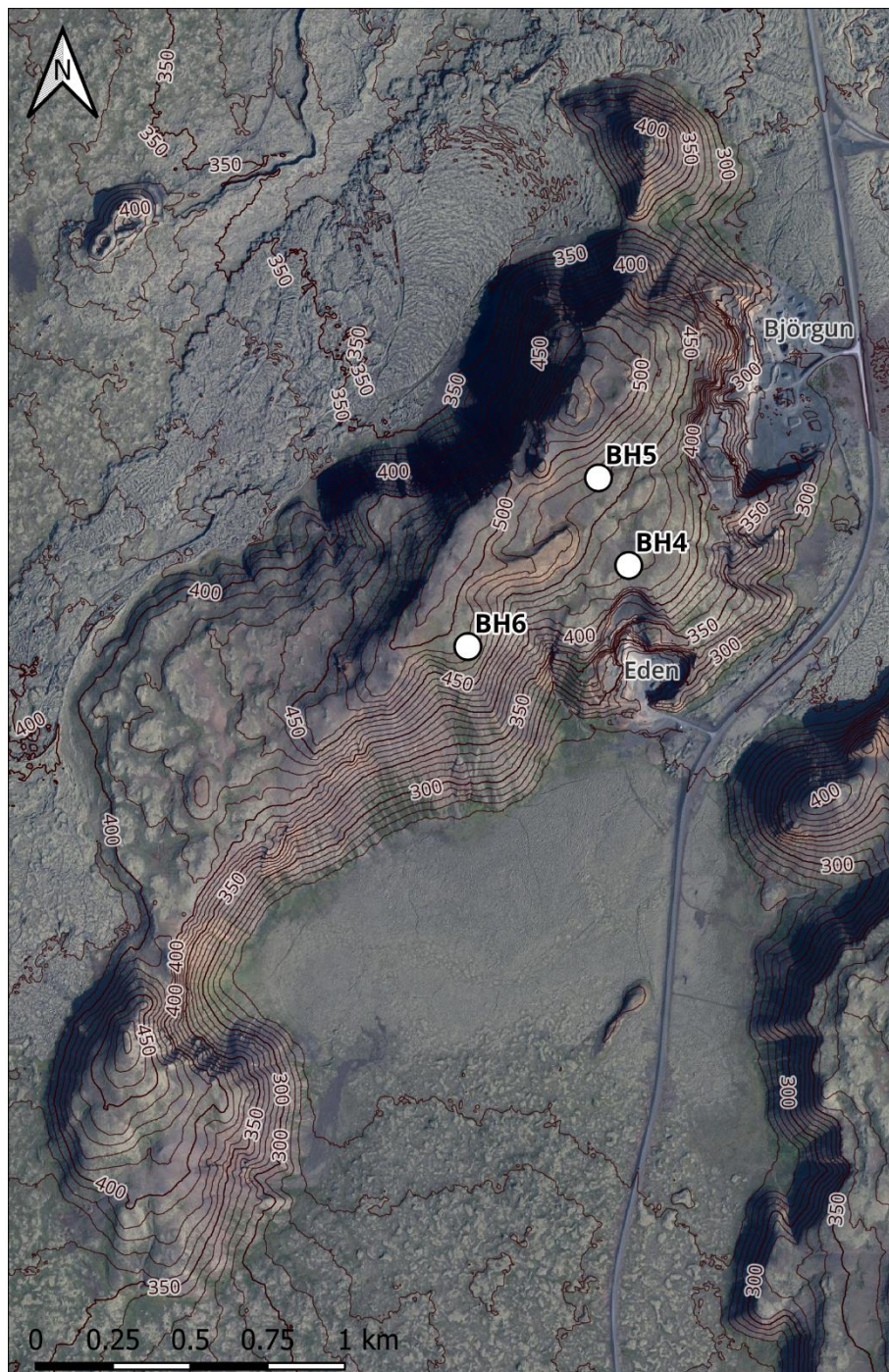
Figure 4 Location of boreholes four to six, drilled into Lambafell to verify the stratigraphy of the material forming the mountain. The orthomosaic and contour lines are sourced from Loftmyndir ehf. and Landmælingar Íslands, respectively.
