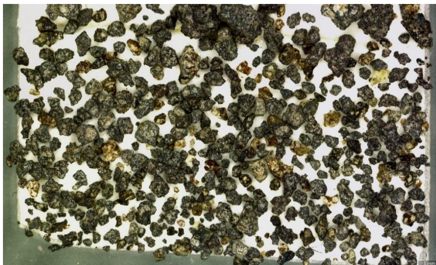
Figure 125 The <1 mm sample is the same as 1 mm. Only two to three loose crystals, PLAG and OL.
