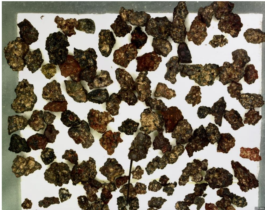
Figure 132 The 1 mm sample contains only crystalline grains and only a few of them are dark gray, almost all of them seem to be orange red, deep red, or have some red in them. Only a handful of black grains have vitreous surfaces but none of them are pure glass. No obvious minerals.
