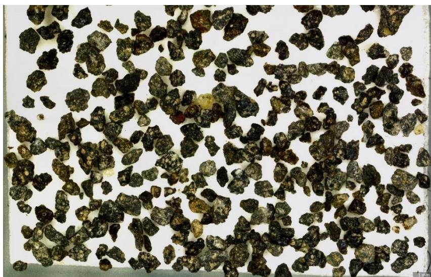
Figure 117 The <1 mm sample is the same as 1 mm. A few red grains. Three loose light yellow to yellow crystals (PLAG and/or OL). Some glass grains seemingly without phenocrysts are present.
