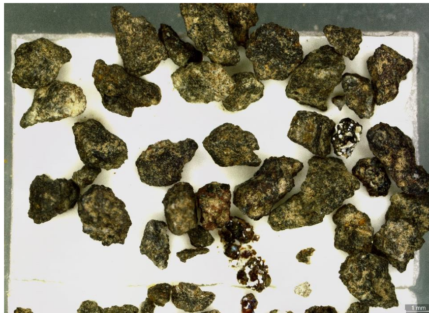
Figure 98 In the 1 mm sample there is light yellow alteration on most crystalline grains (~90%). Some PLAG is present in a few grains, no obvious OL. The glassy grains (~10%) have white opaque minerals within them and one crystal that is likely OL. Some grains are partly red.
