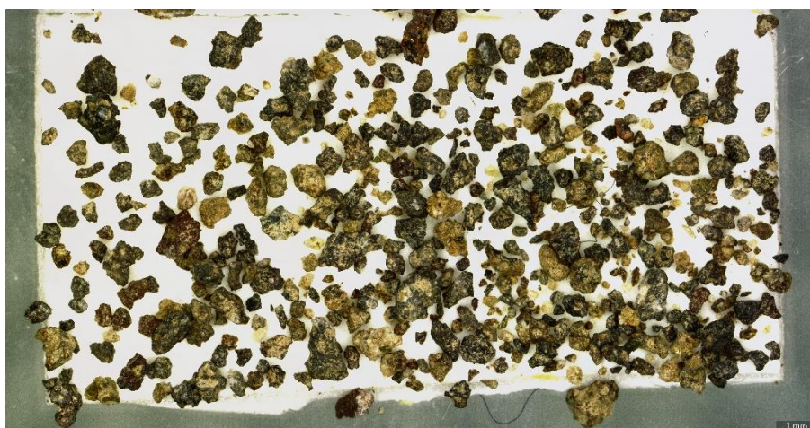
Figure 101 In the <1 mm sample there are some grains completely red with crystals and/or light yellow alteration. Minerals present are OL and PLAG. No clean glass.
