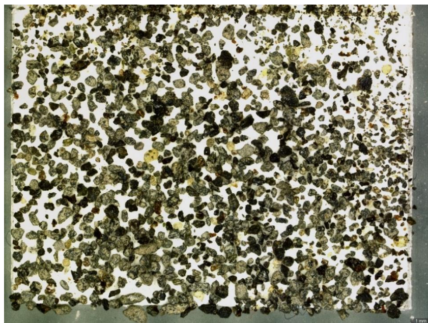
Figure 119 In the <1 mm sample the alteration coating is thinner than in 1 mm. Many black grains are vitreous. There are a few loose PLAG and OL (clear to light yellow to green). Some orange/red grains are present.
