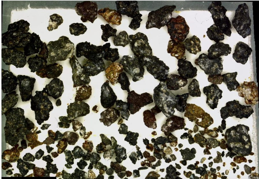
Figure 108 In the 1 mm sample there are more black or dark gray grains (70%), but no pure glass. PLAG and OL present in black grains. Some orange grains (~10%) with opaque minerals along with PLAG and OL. Some dark red grains (~10%) with minerals (at least PLAG). Crystalline grains with a coarse groundmass (~10%) are also present, with a slight green tint. One completely altered grain (brownish yellow). Others are undefined.
