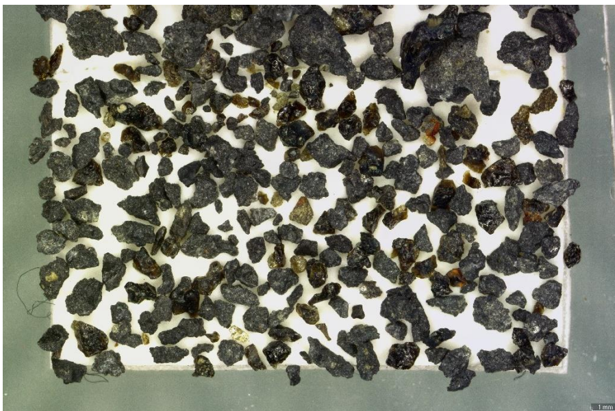
Figure 31 In the <1 mm sample there is more glass than in 1 mm (20-25%). Some grains have rust colored alteration. Few loose crystals.
