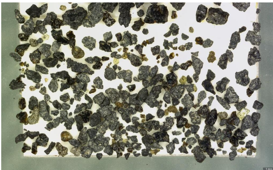
Figure 21 The <1 mm sample is the same as 1 mm. Vesicle rich, golden brown glass present. Some OL and PLAG (<1%).
