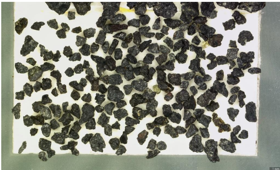
Figure 15 The <1 mm sample is the same as 1 mm. 2-3 grains have patches of reddish surfaces. Only two loose crystals (OL and PLAG).
