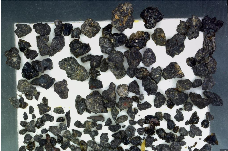
Figure 50 In the 1 mm sample there are mostly crystalline grains (~80%), some slightly altered, most not. A few more glass grains than before (~20%). One glass grain with very large phenocrysts (PLAG), others have some visible phenocrysts (OL and PLAG). A few crystalline grains have obvious phenocrysts (mostly OL), other grains have phenocrysts, but they are difficult to distinguish.
