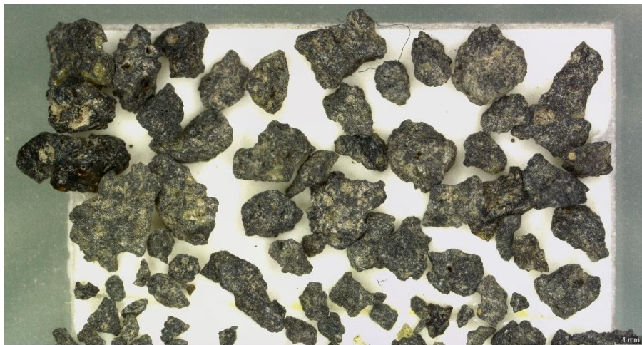
Figure 22 In the 1 mm sample there are only three or four fairly altered glass grains (10%), one is less altered. A few black crystalline grains (~30%) but some are hard to distinguish from the gray coarse crystalline grains (~60%) so their proportions are unclear. OL and some PLAG phenocrysts. White/light colored alteration present in some grains.
