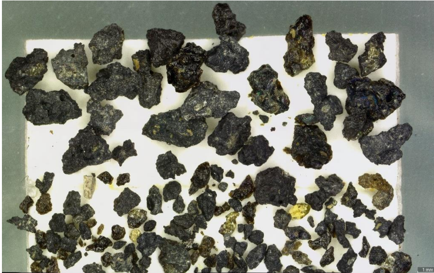
Figure 24 In the 1 mm sample the grains are darker than in BH4-9. Proper glass grains with phenocrysts and slight alteration (~20%), black crystalline grains with phenocrysts and slight alteration (~60%), and dark crystalline grains with phenocrysts and coarser groundmass (20%).
