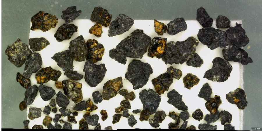
Figure 6 In the 1 mm sample there are mostly crystalline grains (~75%) but some altered glass is present (~25%). Alteration is dark yellow to orange, mostly in vesicles or cavities. Some PLAG and OL are present in most grains.
