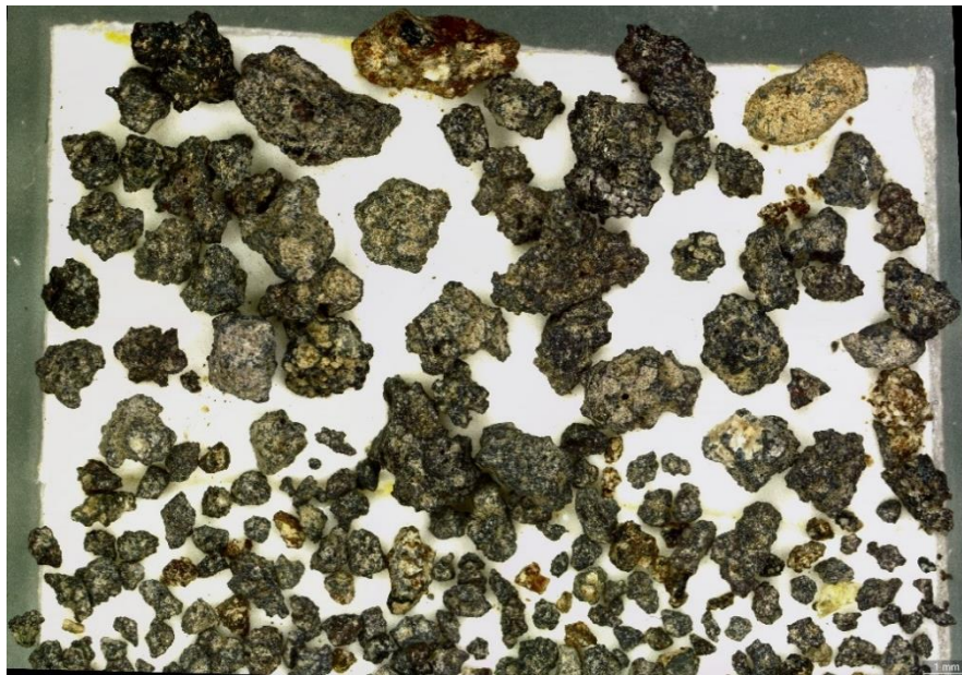
Figure 124 In the 1 mm sample there are mostly crystalline grains (~75%) along with a few glassy grains (~20%), two red grains and one with an altered coating. No phenocrysts to speak of but there is a hint of OL in some grains. The red grains and one crystalline grain contain white opaque minerals.
