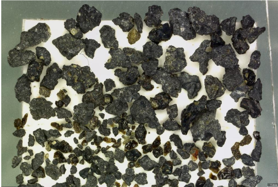
Figure 30 In the 1 mm sample there is less glass (~15%) again and one golden colored grain covered in easily altered ground glass, otherwise dark crystalline grains with some phenocrysts (OL and PLAG).
