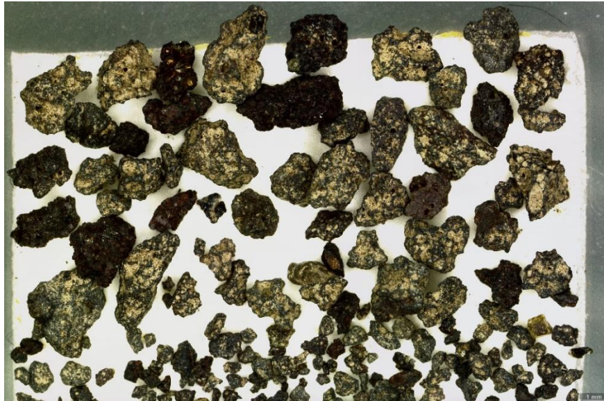
Figure 126 In the 1 mm sample there are mostly crystalline grains (~55%; some reddish), some black vitreous grains (~25%), and some dark red vitreous grains (~20%). All types have both altered and non-altered grains, but most grains are altered which could obscure the distinction between grain types. One obvious OL phenocryst, no white opaque minerals.
